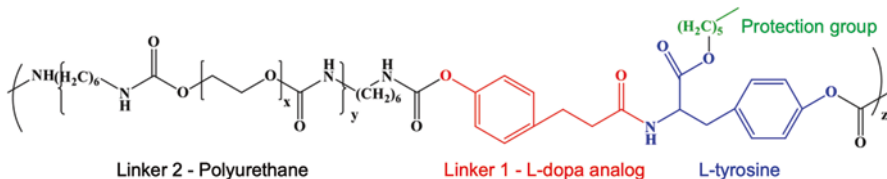
Fig. 4 Chemical structure of L-tyrosine polyurethane. L-tyrosine is modified with L-dopa analog and polyurethane linkages
