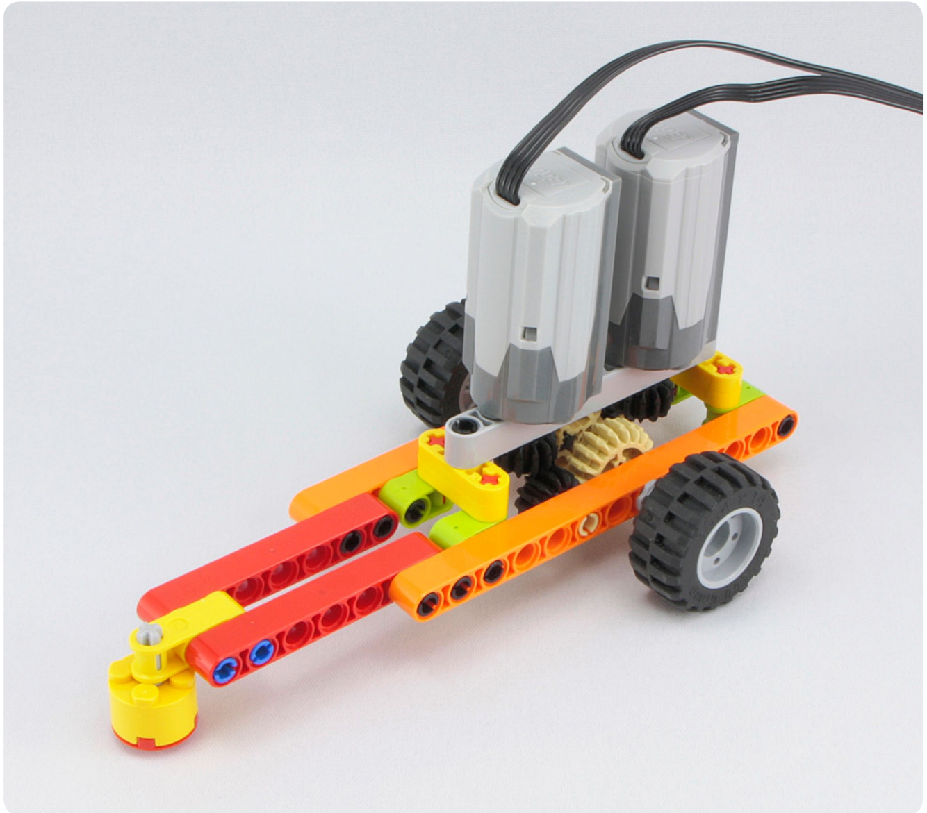
42 Each motor turns a wheel
