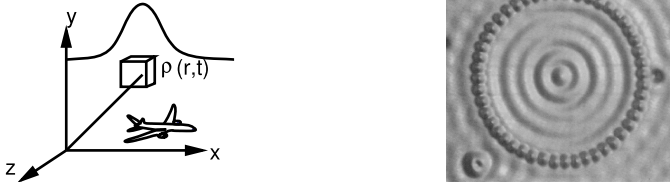
Figure 1.2: (Left) Quantum probability density \rho(\mathbf{r}, t) . (Right) Experimental scanning tunneling microscope spatial image of the surface states of the electron in a quantum corral of 48 Fe atoms [9]. Used with permission from AAAS.
