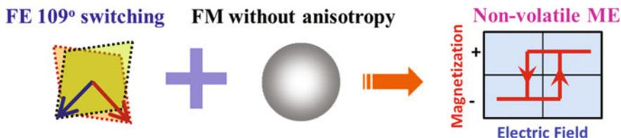
**Fig. 3.22** The mechanism summary of the nonvolatile electrical control of magnetization
