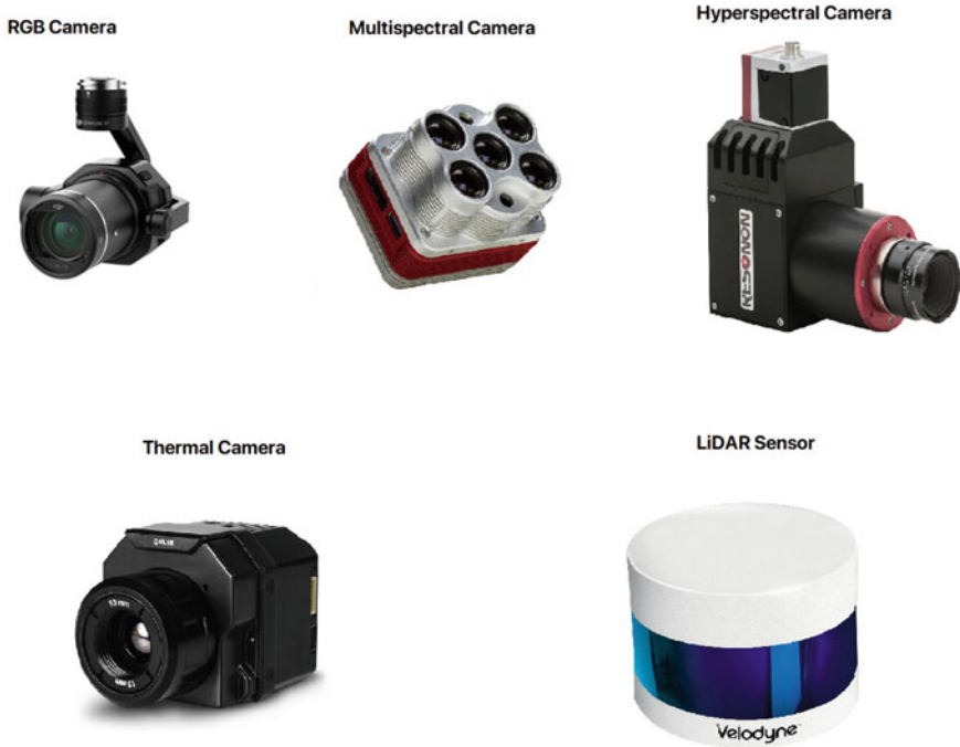
Fig. 1.2 Different types of sensors outfitted to UAVs
