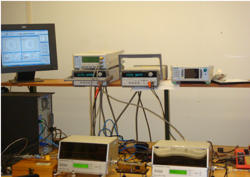
Figure 10. Load-pull bench used to characterize the device
