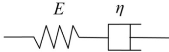
Figure 3. Maxwell model consists of a viscous damper \eta and an elastic spring E connected in series.
