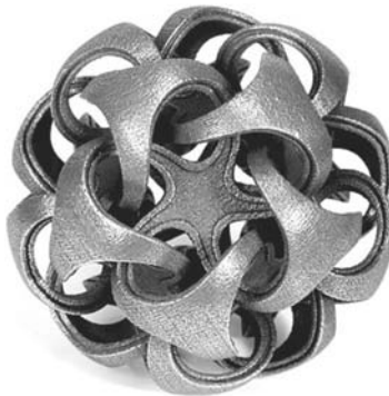
Figure 6.7 Quintrion, metal print sculpture. Note the geometric complexity and nested shapes achievable with RP. (Courtesy of Bathsheba Grossman.)
