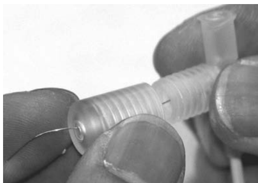
Figure 4.10 Assembling lead screw pull mechanism.
