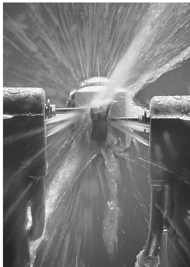
Figure 6.10 Milling the ceramic blank. (Courtesy of Sirona Dental Systems.)
