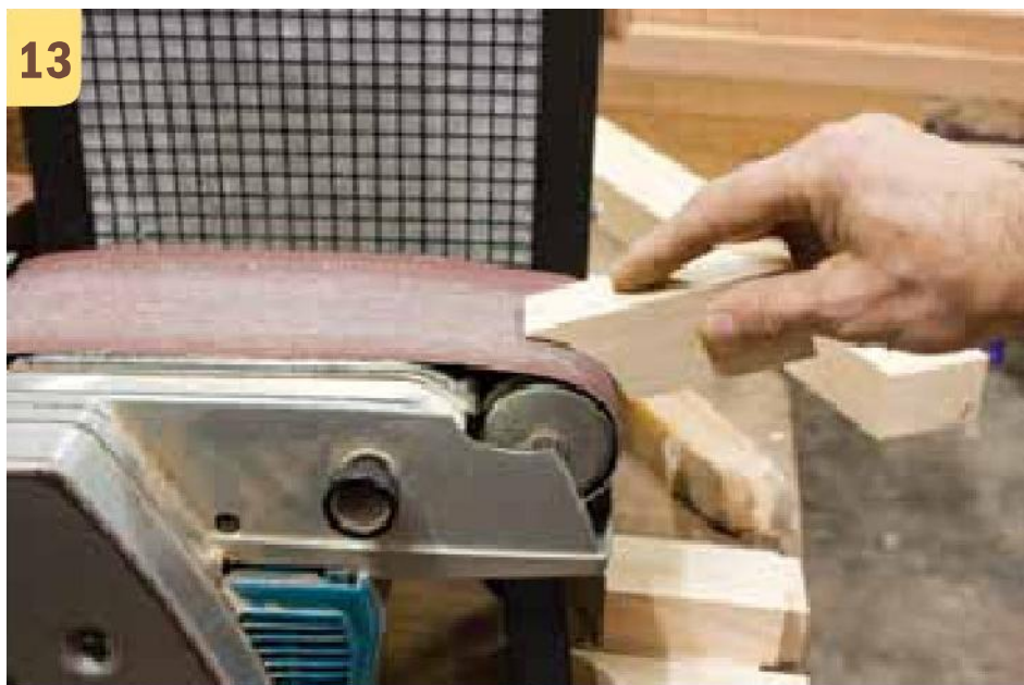
Curved rail supports were sawn and finished on a sander.
