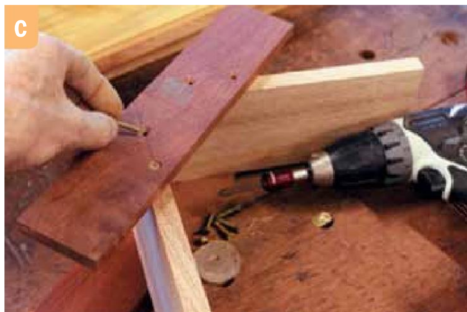
C Use screws to strengthen the sled, but make sure the screws don't foul the sawblade
