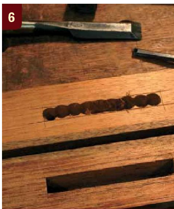
The mortises for the back rail tenons are drilled and then cleaned out with a chisel.
