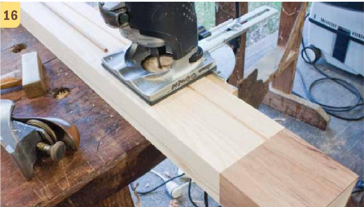
A groove was routed on the outside leg faces.
