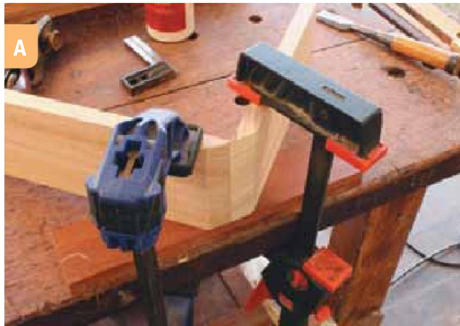
A With the components sawn to length glue one half of the sled together.
