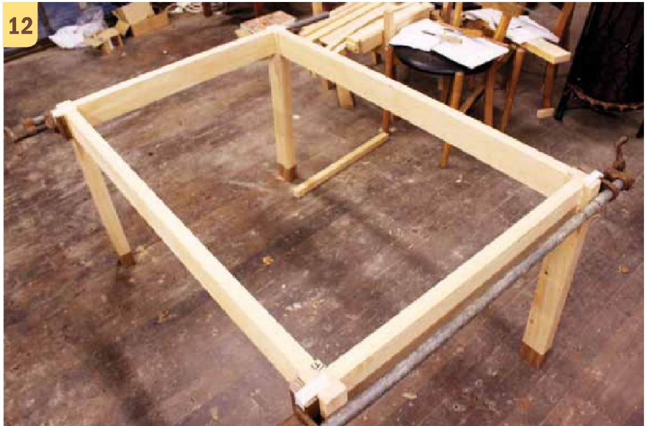
The short rails are glued in place and the whole frame checked for square.
