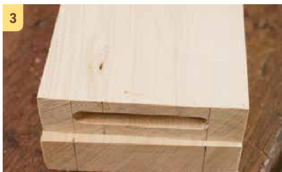
Leg to rail joint, in this case a floating mortise and tenon.
