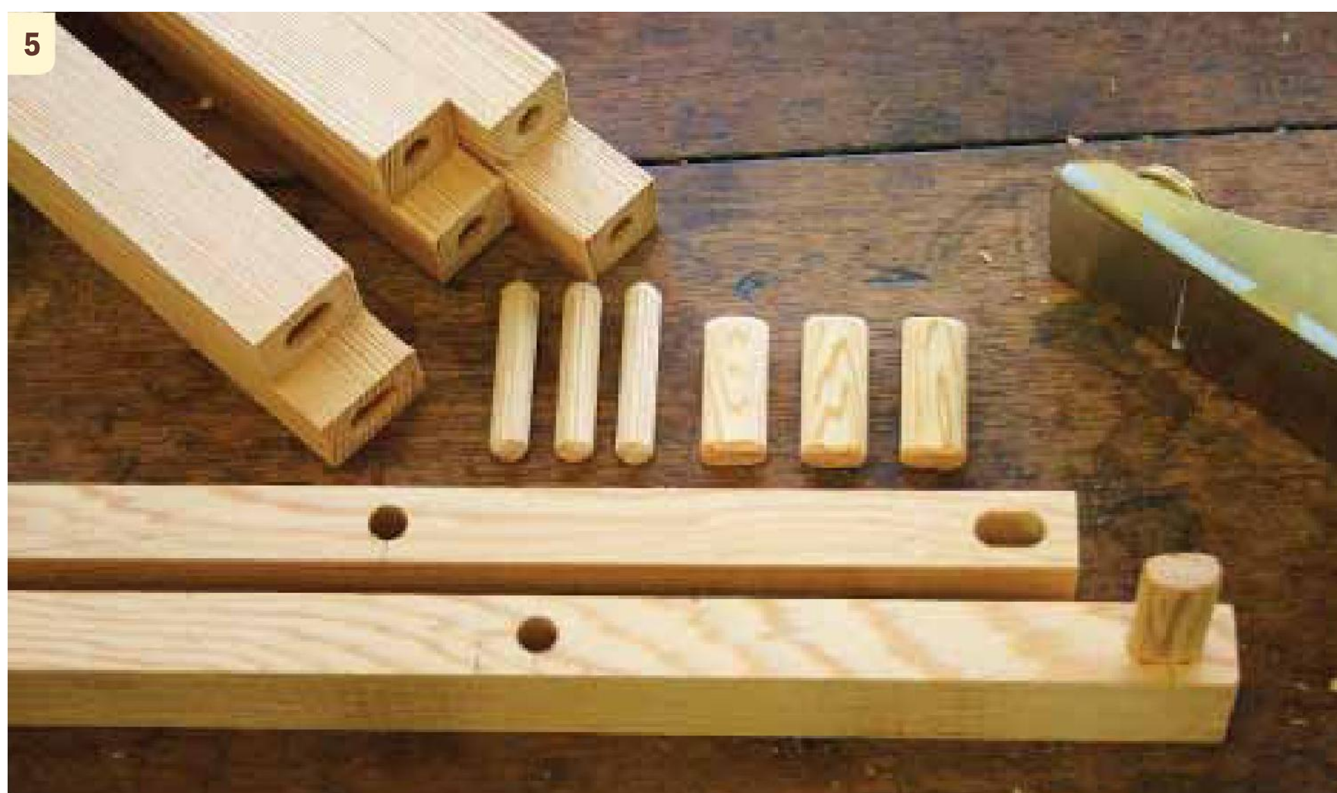
The door use small floating tenons at the corners and dowels for the centre rails.
