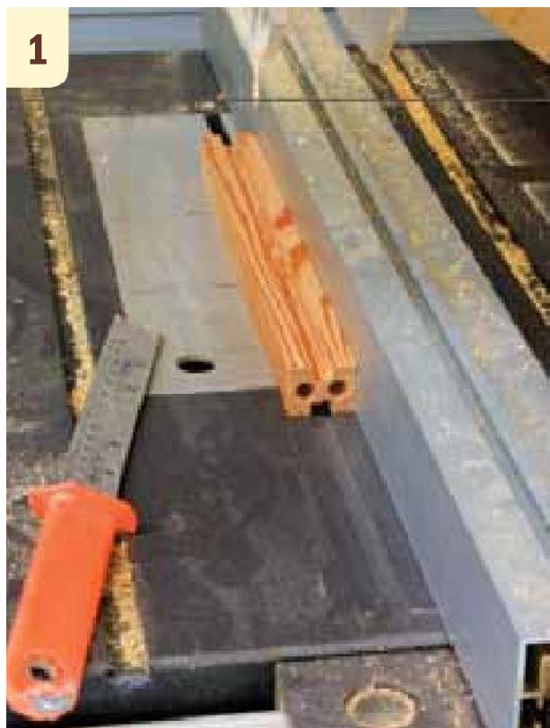
1 Sawing grooves in the frame components on the panel saw. Always use pushsticks when working at the tablesaw.
