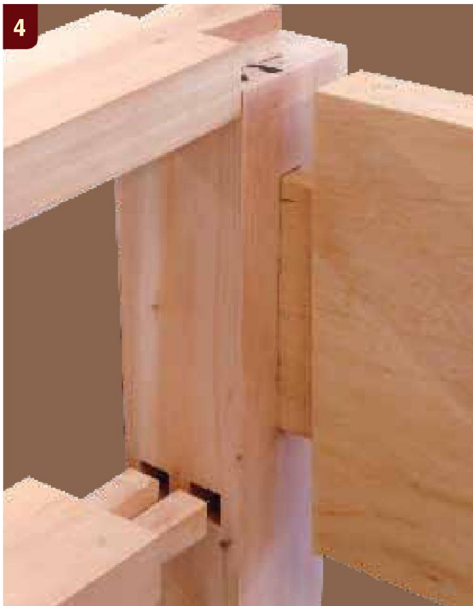
Front leg joints. Lapped dovetail at top and twin stub tenons. The side rail has a large tenon. The lower rail yet to be sawn down to meet the leg curve.
