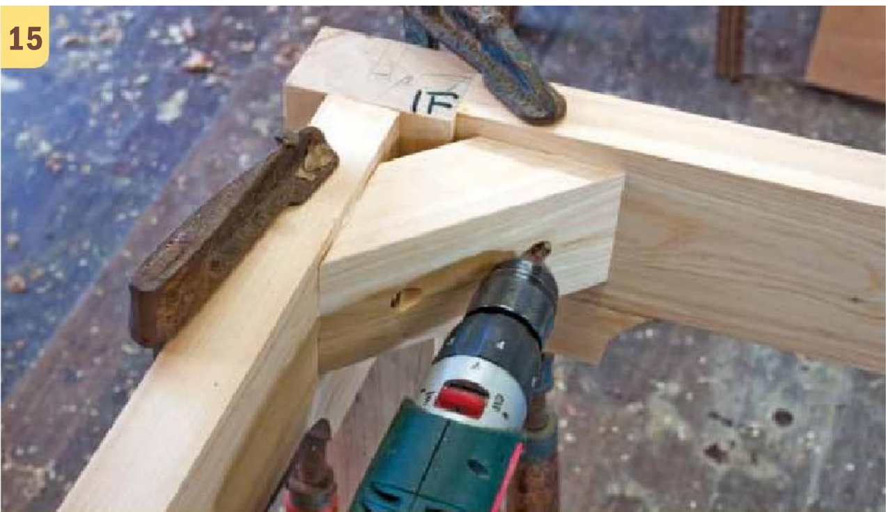
Mitred blocks are glued and screwed into the frame corners to strengthen the frame.
