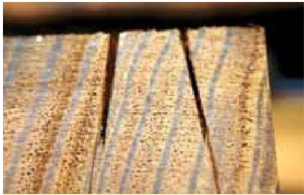
The cut on the right is too close to the knife line. The left cut is much better as it leaves the line intact.
