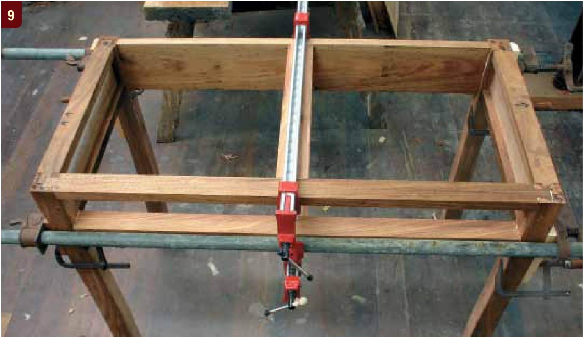
The desk front and back are glued to the sides. Note how the centre drawer runner and kicker are glued in at the same time.
