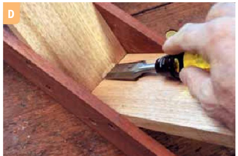
D The 'mouth' of the sled will need to be carefully opened up with a chisel.
