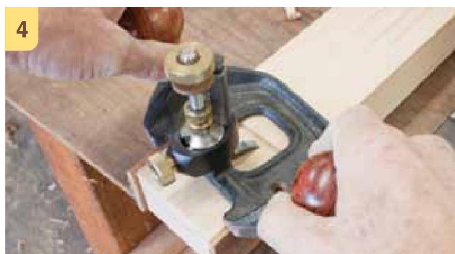
Using a router plane to clean up the recess for the blackwood feet.
