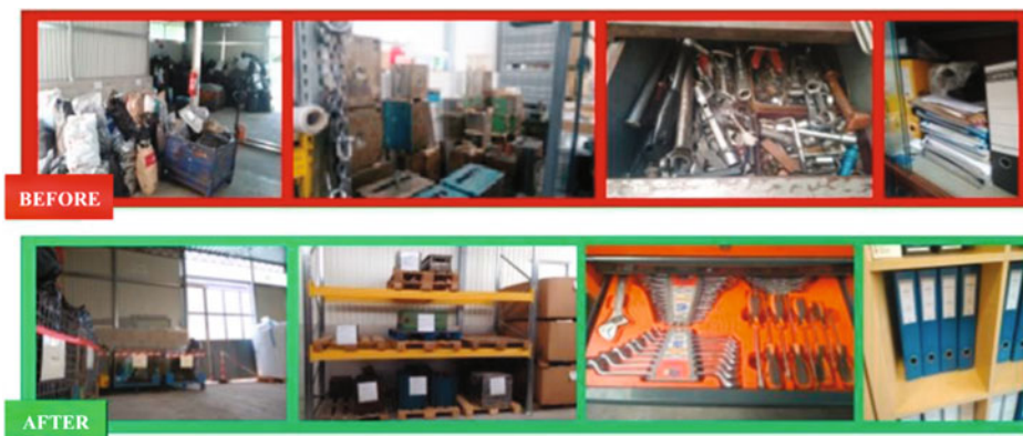
Fig. 1.9 Example of application of the 5's in a plastic products manufacturing plant [32]
