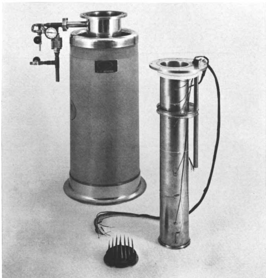
REFERENCE SOURCE ( foreground ) for the Princeton radiometer is made of metal-coated fiber-glass spikes. It has been removed from the Dewar flask and the pipelike wave guide that is normally coupled to the antenna horn. Wires on wave guide lead to thermocouples.
