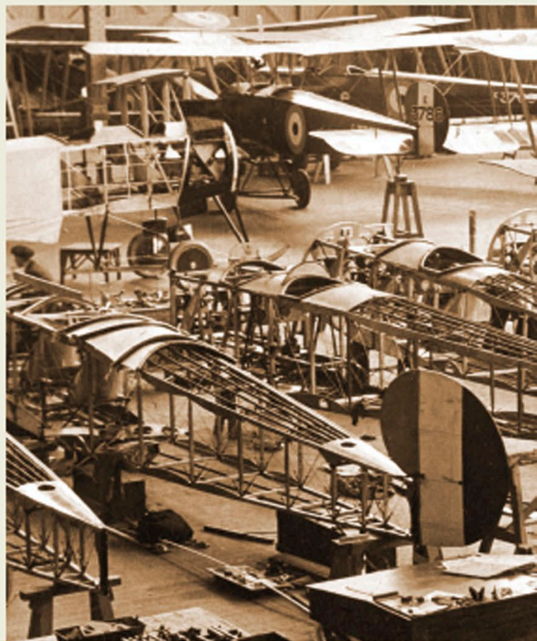
Avro 504 biplanes being manufactured at a factory in Hampshire, England, during World War I
