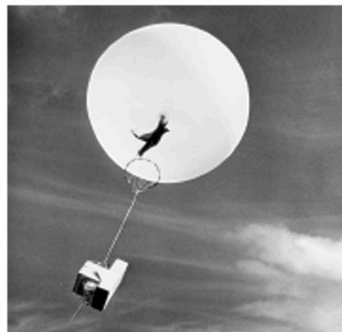
Weather balloon with a radiosonde attached
