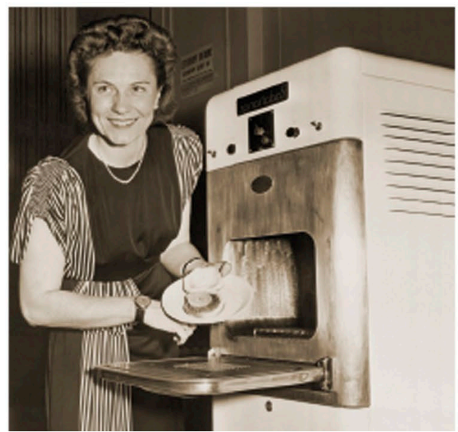
Hamburger cooked in an original Raytheon Radarange microwave oven
