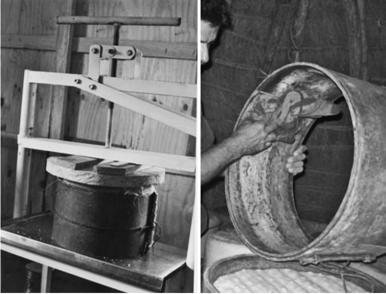
Figure 5.3 Cotija press and a worker cleaning the belt used for molding the cheese
