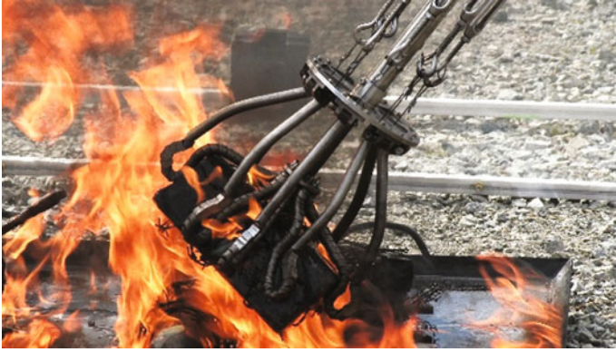
Fig. 2.14 Fire-resistant gripper mechanism equipped with a flexible and rigid switchable linear body (Tadakuma et al. 2008)
