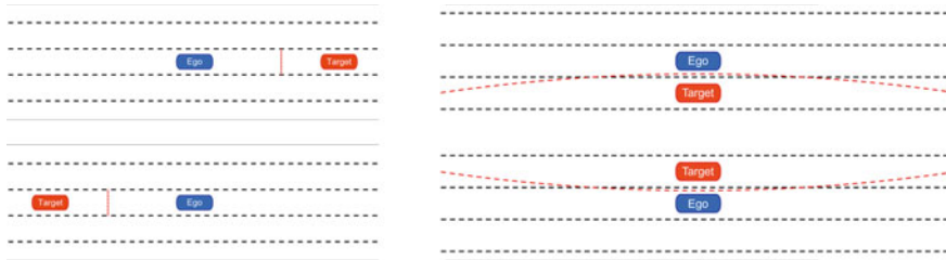
Fig. 15 Longitudinal and lateral barriers
