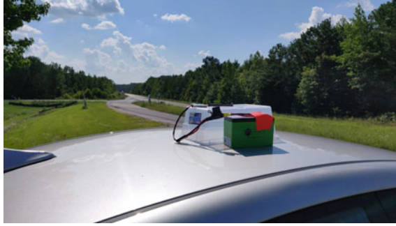
Fig. 31 Interference source (28 dBm) placed adjacent to the test track at NCAT
