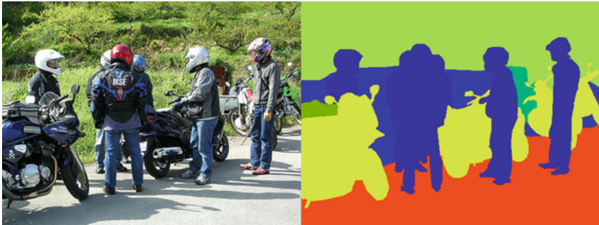
Fig. 20 An instance of semantic segmentation
