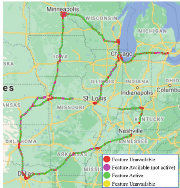
Fig. 8 Map Data ©2021 Google. Actual feature experience for a development drive relative to the ADAS feature availability map
