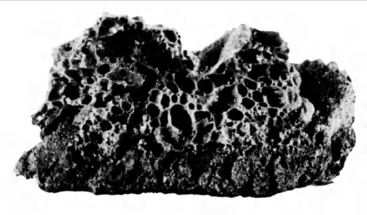
Figure 2. Slagging deposit showing segregated development.
