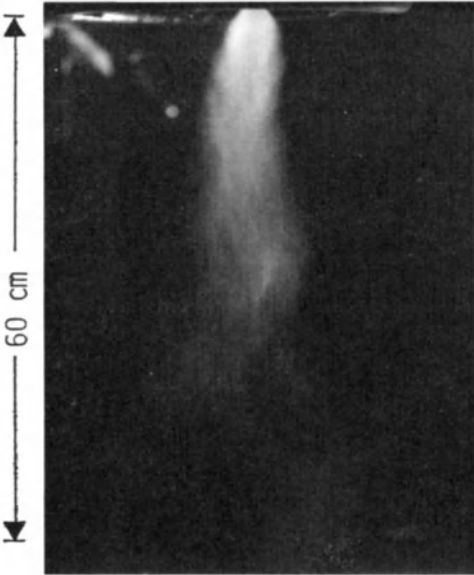
Figure 9. Hexane Spray Pattern and Flame for 34 PSI Atomizing Air Pressure (a and b) and 60 PSI Atomizing Air Pressure (c and d). a and c) Spray - No Flame, b and d) Flame at 1/1000 sec. Shutter Speed.
