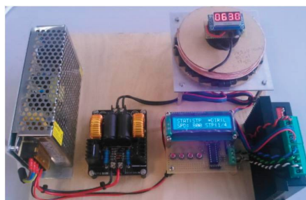
Figure 8. A PI with ED that was used for the realization of a contactless charging station of a motoped.
