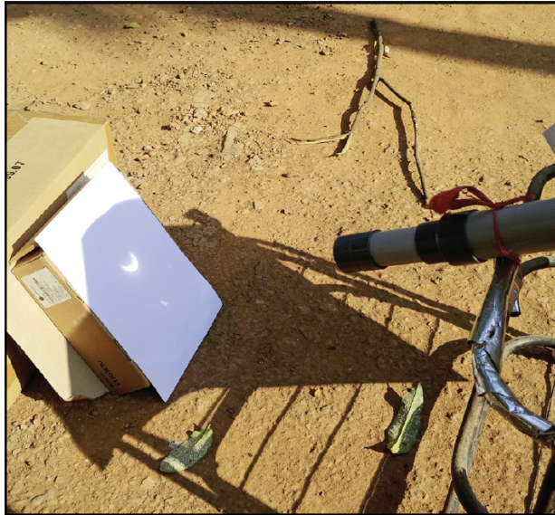
Solar projection method used to watch a partial solar eclipse.
