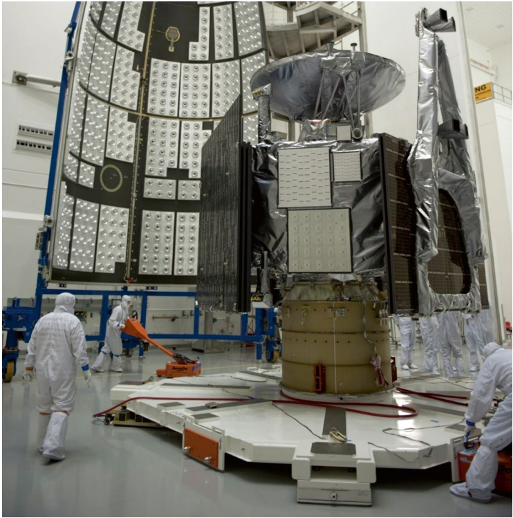
Fig. 9.14 Juno spacecraft showing five antennas for the microwave radiometer (NASA photograph cropped by author)
