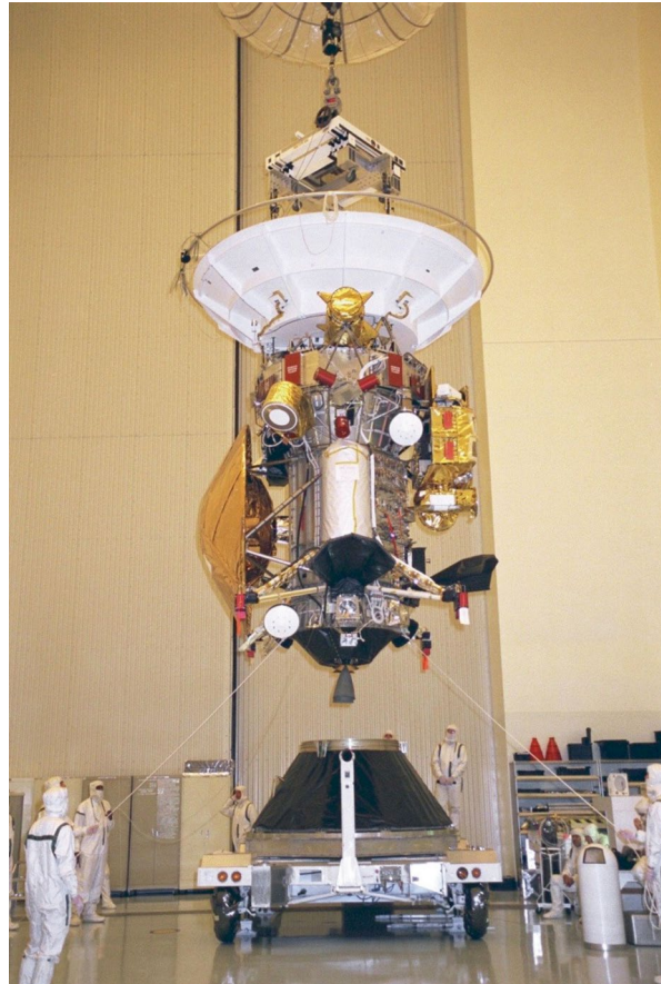
Fig. 6.2 Cassini-Huygens being mated with launch adapter. (NASA photo)
