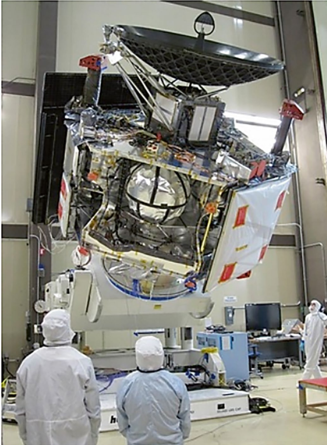
Fig. 9.3 View of Juno with two solar panels removed (NASA image)
