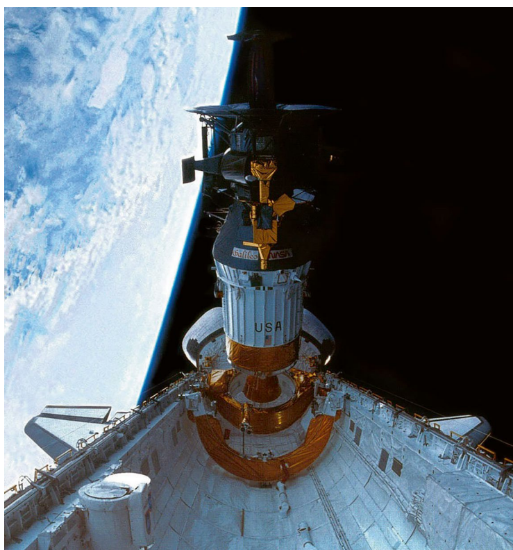
Fig. 7.5 Galileo spacecraft and inertial upper stage booster raised to launch position in cargo bay of Space Shuttle Atlantis (NASA image)
