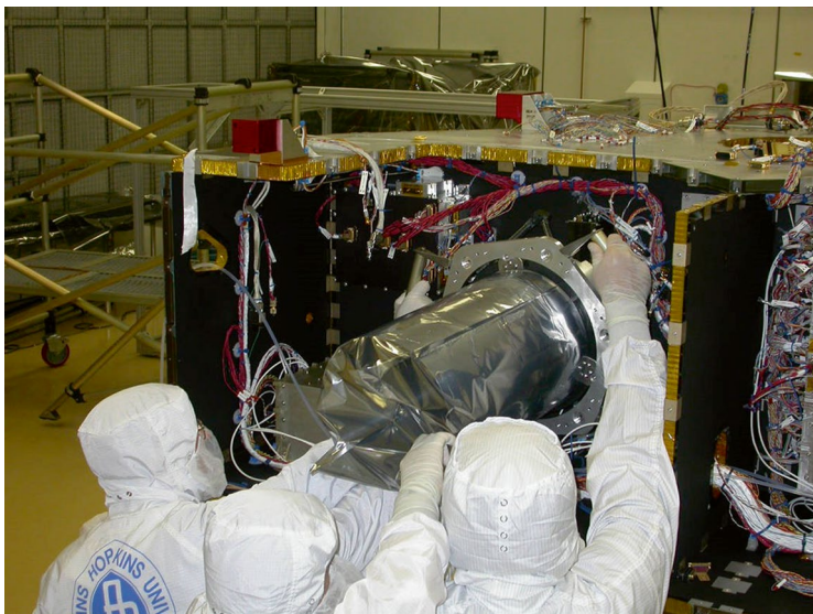
Fig. 8.8 Installation of LORRI on spacecraft (NASA photograph)
