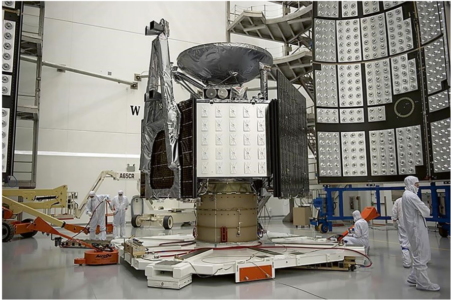
Fig. 9.13 Juno spacecraft showing the antenna for the 0.60 GHz microwave radiometer channel (NASA image)
