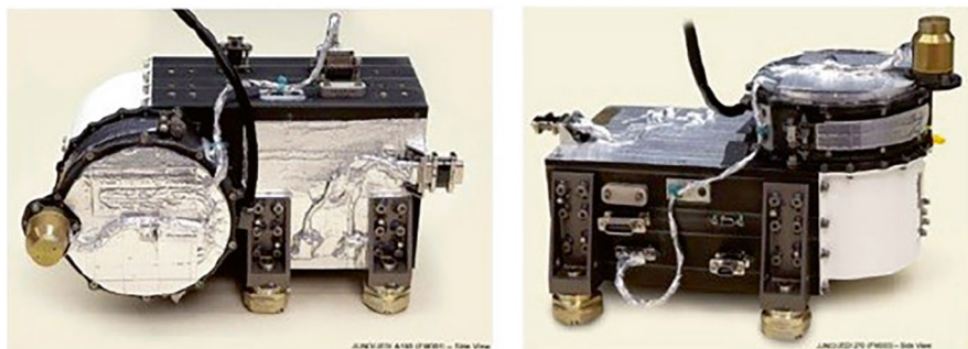
Fig. 9.19 Design of sensor head for Jupiter Energetic Particle Detector Instrument (NASA/JHU image cropped by author)
