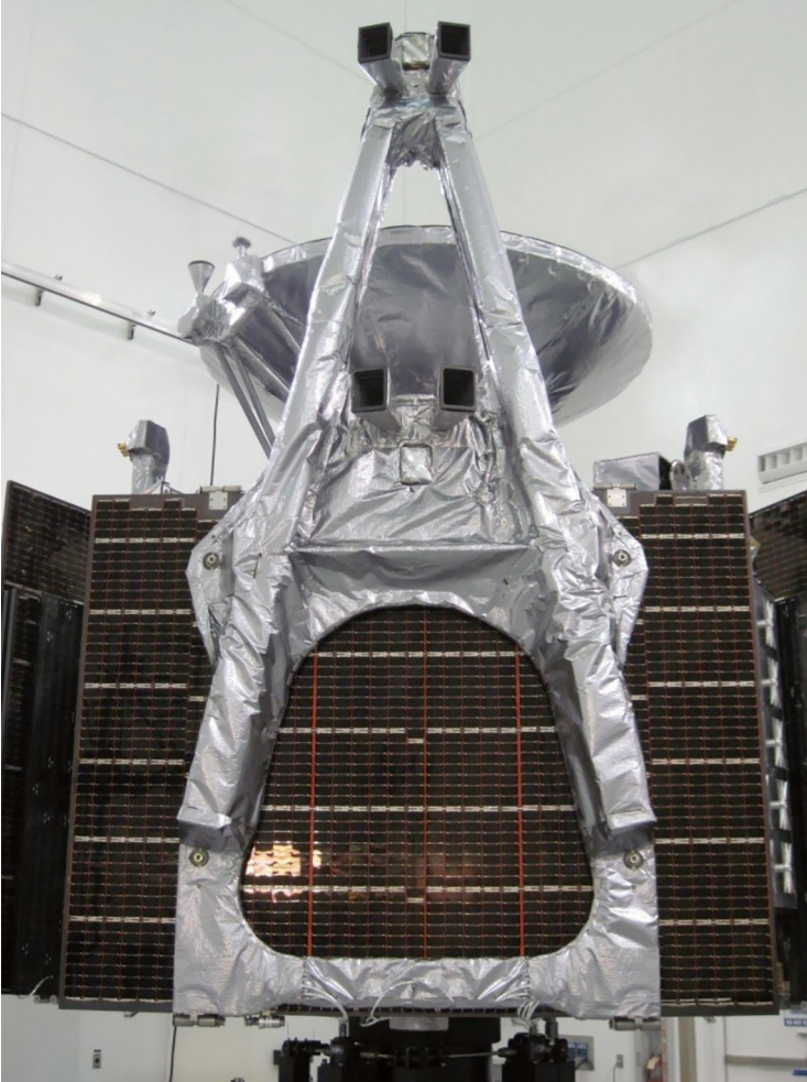
Fig. 9.16 Magnetometer boom in stowed position. (Image credit: NASA/JPL-Caltech/LMSS)
