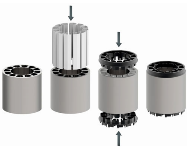
Figure 3.85 Assembly steps for full lamination stacks
