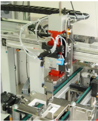
Figure 4.27 Comparison of handling with pneumatic gripper and robot
