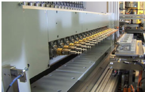
Fully automated linear winding machine with 20 spindles and pivoting frame
