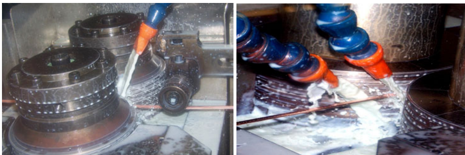
Figure 2.21 Rolling pair for profile wire production (Picture: Essex Germany GMBH)
