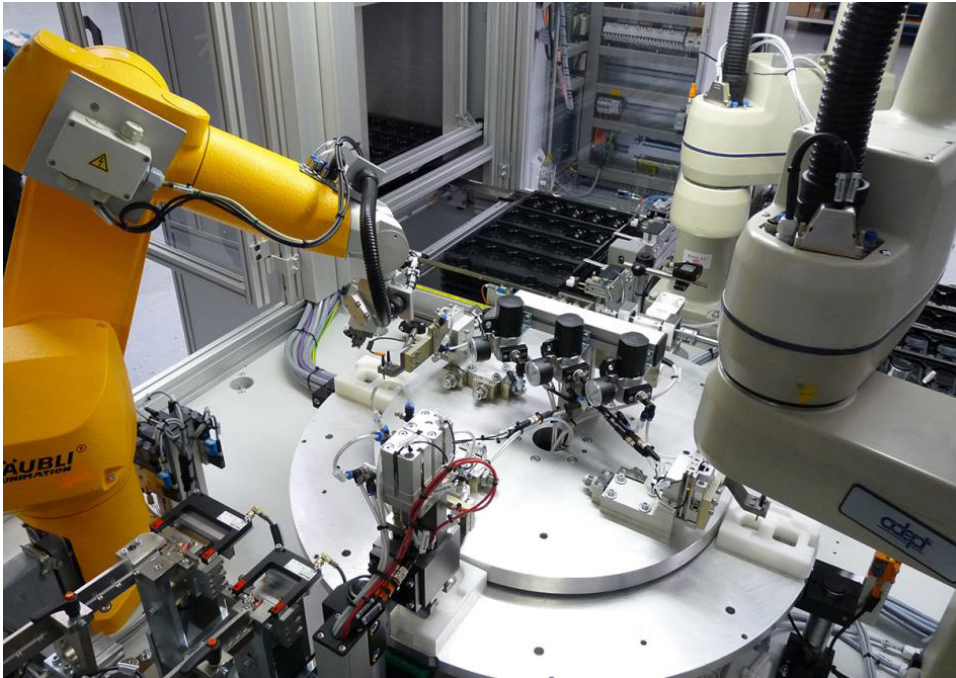
Figure 4.12 Rotary table with robots and palletiser
