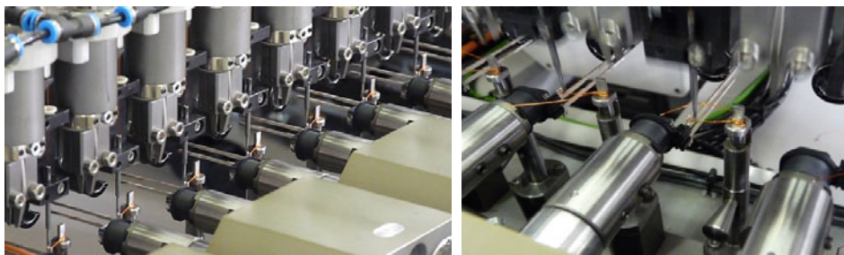
Figure 3.42 Usage of park pins within the machine
