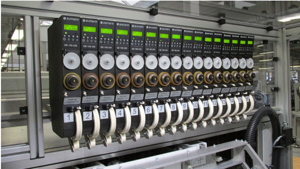
Figure 3.22 Wire tension control systems in winding technology
