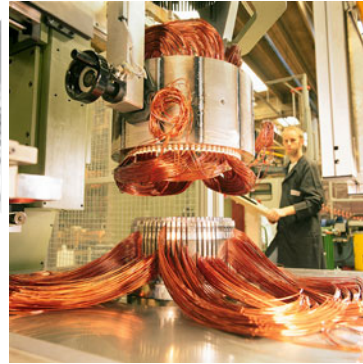
Figure 3.66 Winding preparation according to [Tzs-90]. Picture (right): Otto Rist GmbH
