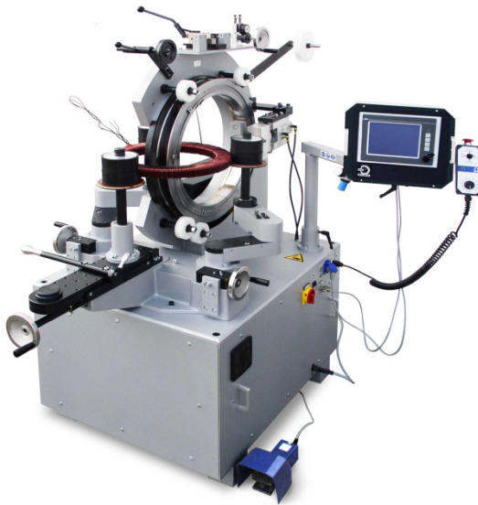
Figure 3.65 Demonstration of the toroidal winding process. Scan QR code to view video demonstration. (Picture: Ruff)
