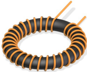
Figure 3.17 Schematics of a toroidal winding
