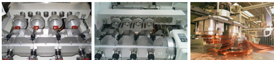
Figure 3.50 Comparison of bell-, disk-, and template flyer (Picture on the right: Otto Rist GmbH & Co. KG)
