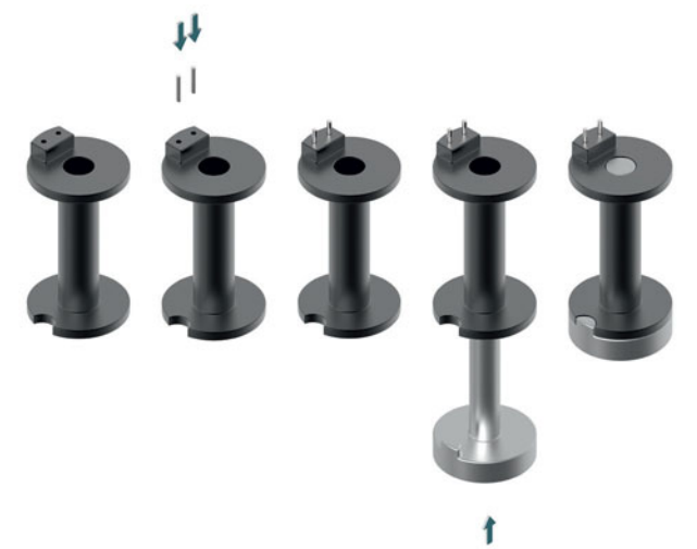
Figure 3.84 Assembly steps for coil bobbins
