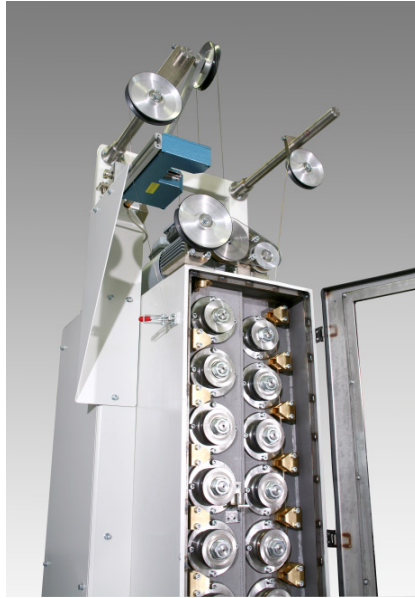
Figure 2.20 Complete setup of a wire drawing unit
