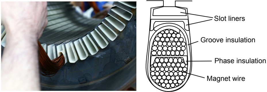
Figure 3.71 Insulated stator and groove insulation structure [Toliyat 2004]
