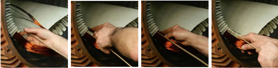
Figure 3.75 Feeding of outer strands
