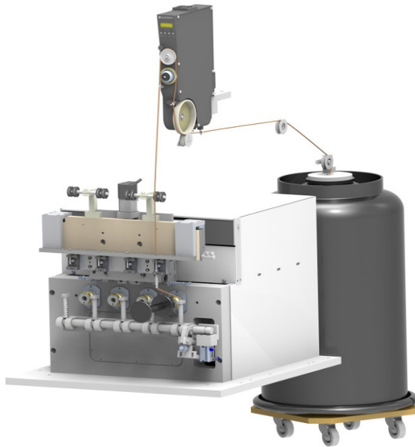
Figure 3.38 Wire path in a linear winding machine
