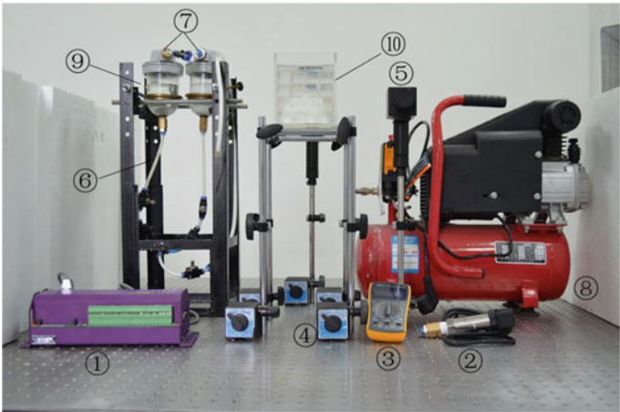
①digital acquisition instrument; ②pressure transducer; ③multimeter; ④magnetic holder; ⑤CCD camera; ⑥grouting pipe; ⑦air inlet; ⑧air compressor; ⑨grout container; ⑩transparent rock model
