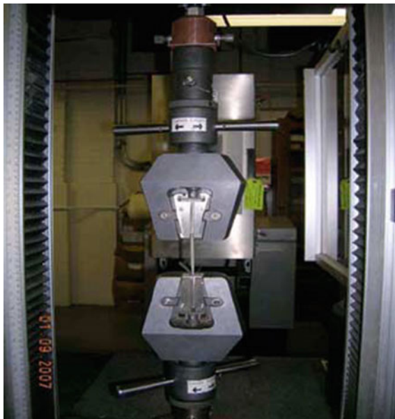
Fig. 6.4 The experimental set up for the tensile test of the latex membrane
