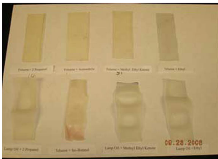
Fig. 6.3 The latex membrane 40 h after the immersion test
