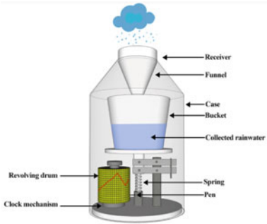
(a) Weighing bucket-type rain gauge
