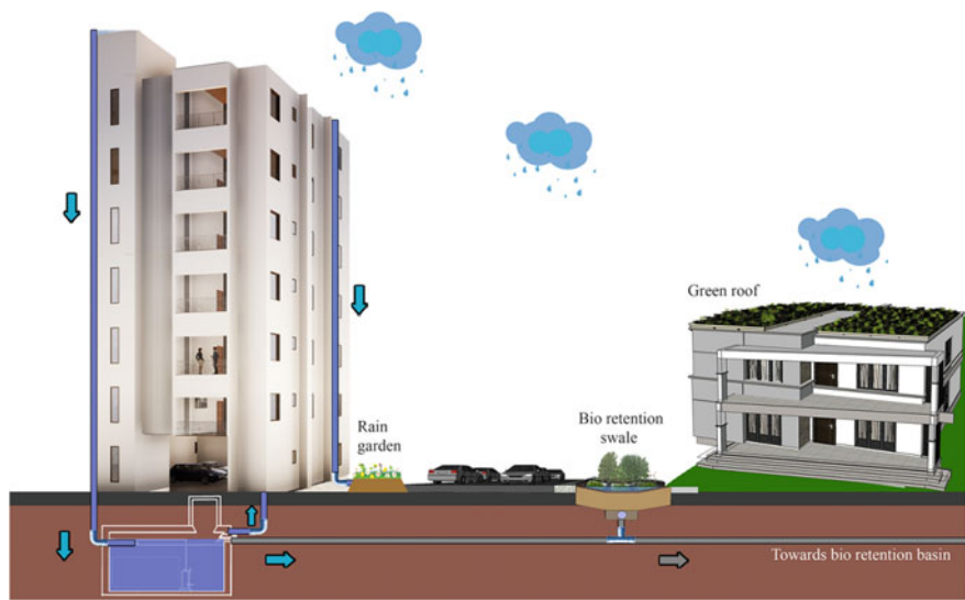
Fig. 4.16 Rainwater harvesting system for stormwater management
