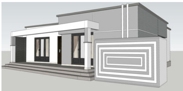
(a) Above ground (away from the building) rainwater storage
