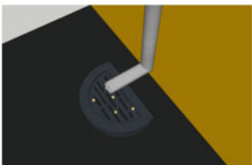
(c) Downspout filters prevent debris from entering the tank
