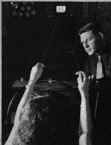
Manipulation of strings helps the inspector test driver's judgment of depth and distance.
