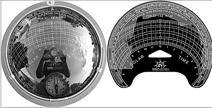
Figure 2.19 Final output of Solar Pathfinder at a given site. (Source: Refer Annex. A)
