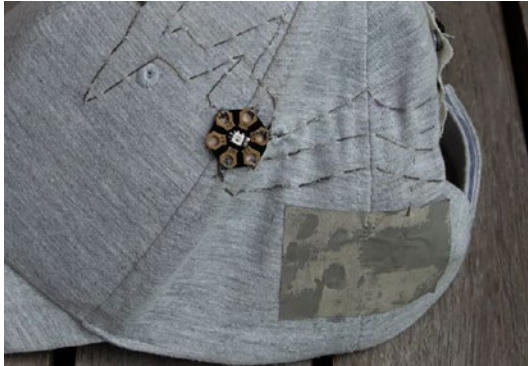
Figure 4-36. All the connections replaced with sewn lines
