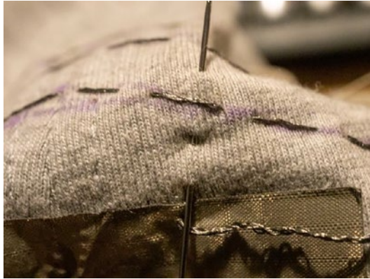
Figure 4-34. Sewing under another line to prevent short circuits
