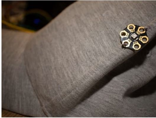
Figure 4-24. Positioning and orientation of the first LED on cap seam
