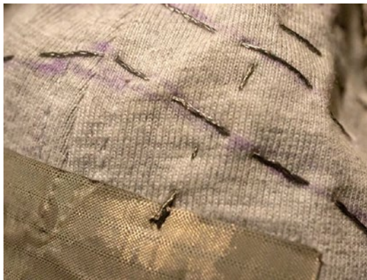
Figure 4-35. The finished sewn lines, crossing without shorting
