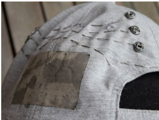
Figure 4-37. Connecting to the press studs
