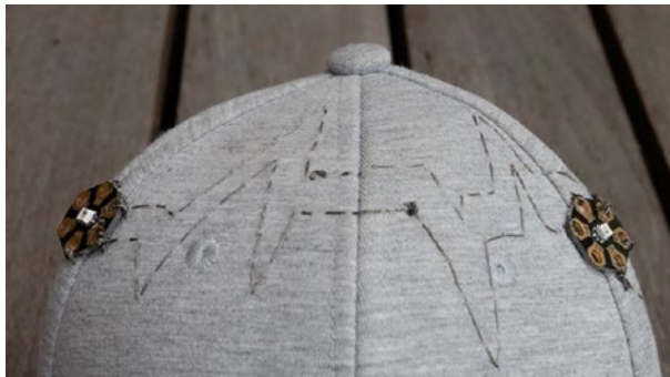
Figure 4-28. Both LEDs connected (two external connections and one internal connection)
