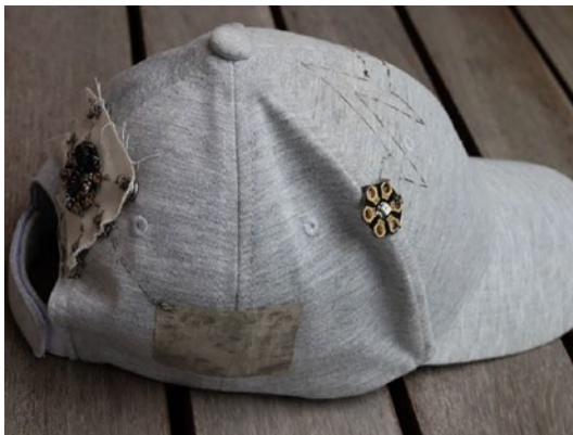
Figure 4-33. Conductive fabric square glued in place with conductive thread connection to Gemma
