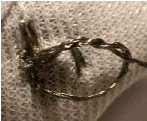
Figure 4-11. Tying off, ready to tighten
