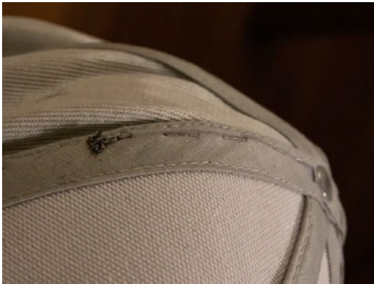
Figure 4-26. Internal connection between LEDs ( out to in )
