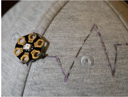
Figure 4-27. LED connection on the outside of a cap (gnd to gnd)
