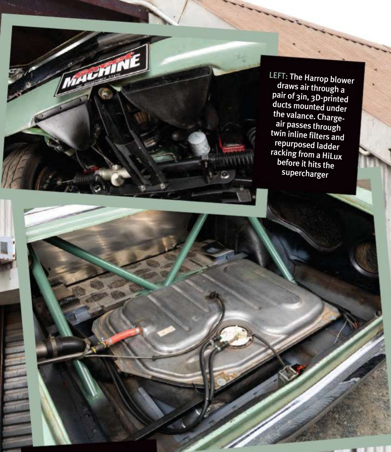
FUEL TANK: Rather than going through the expense of building a custom tank or fuel cell, James cut out the HK's stock spare wheelwell and fuel tank and replaced them with the donor VR Commodore's set-up. An in-tank Walbro 460Lph pump provides plenty of go-sauce to the hungry 5.0L up front
