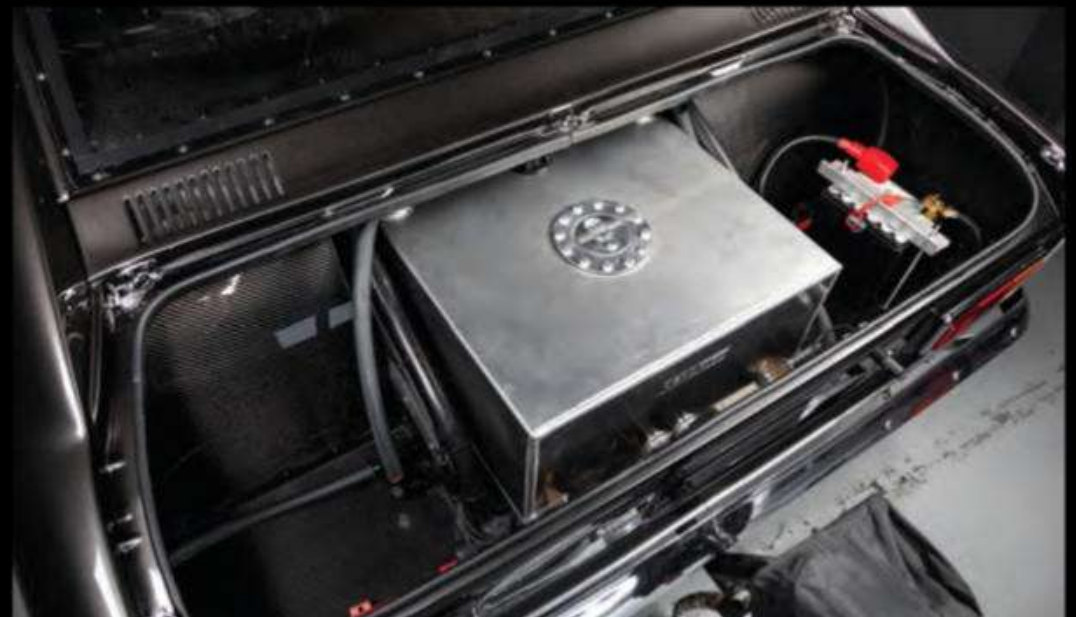
BOOT: Nestled between the gargantuan carbonfibre tubs is a 60L fuel cell. That'll be needed for the road miles on Drag Challenge, while Al switches to VP Racing fuel at the strip
