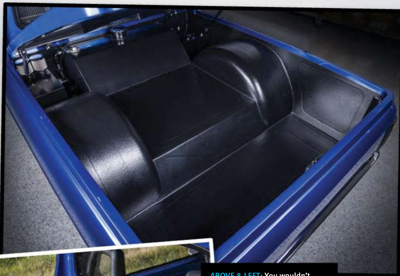
ABOVE & LEFT: You wouldn't think there'd be much room left for ute activities after tubbing a little 1200 to take 19x13 Simmons wheels, but there is! The neat tub job is hidden under an aluminium hardlid, handmade in-house by SR&C boss Shane Rowe
