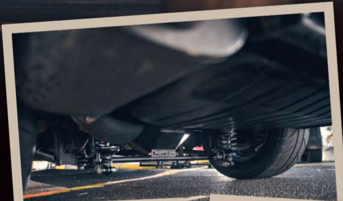
ABOVE: Mark used a spare pair of wheel tubs from a donor Commodore to make the split tubs Code Brown needed to run race rubber. The rear end employs a sheet-metal gin and coil-overs, both from Gazzard Brothers, with the latter using adjustable AFCO struts
