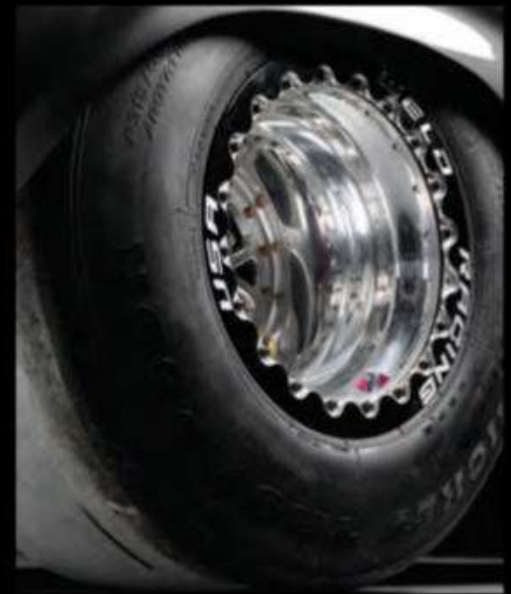
WHEELS: For our photoshoot, the Capri was running Weld V-Series 15x14 rear hoops with 315 radials, but it'll be back on 275s for Drag Challenge 2024 to suit the Radial Aspirated class regs. The 315s will go back on later in the pursuit of quicker ETs
