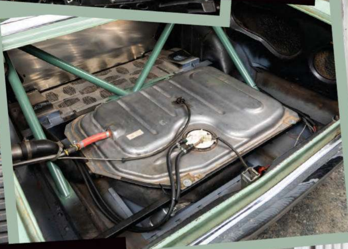
FUEL TANK: Rather than going through the expense of building a custom tank or fuel cell, James cut out the HK's stock spare wheelwell and fuel tank and replaced them with the donor VR Commodore's set-up. An in-tank Walbro 460Lph pump provides plenty of go-sauce to the hungry 5.0L up front
