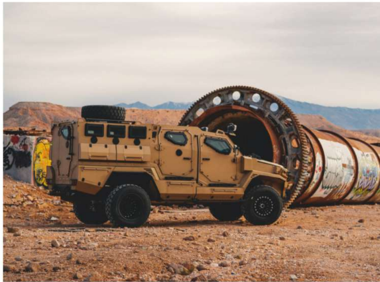
B6 Ballistic Rating standard. Complete 360-degree armored passenger cabin.
