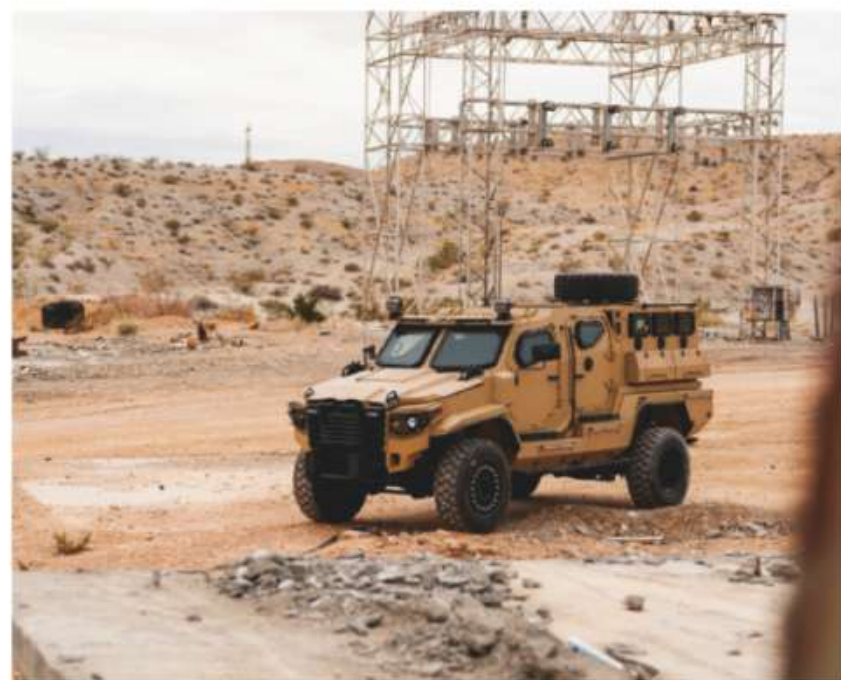
B6 Ballistic Rating standard. Complete 360-degree armored passenger cabin.
