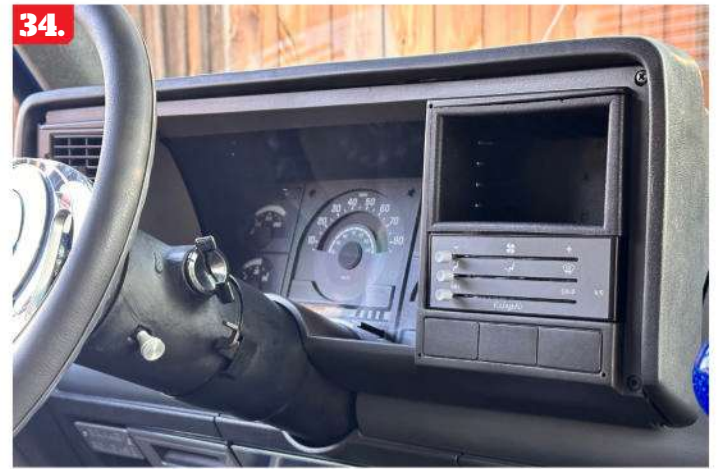
32. Mounting the control panel will be the easiest part of the whole installation—four screws in the stock location. Plug the harness off from the control to the module on the front of the evaporator.
