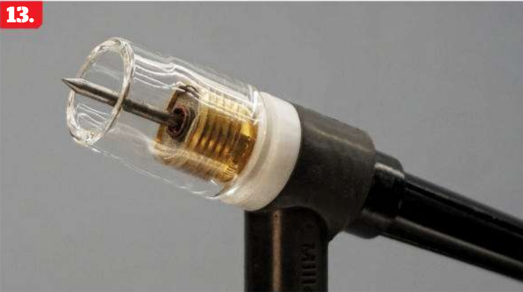
13. There are clear cups available that will brighten the weld area and sometimes give you a better view.
