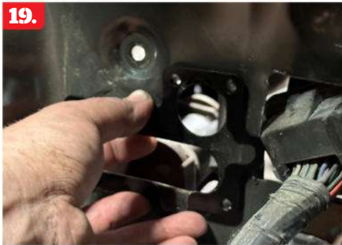
18-19. Using the supplied template, we were able to drill the holes in the required location for the hose and wire exits, despite the firewall tub and wiring harness location.
