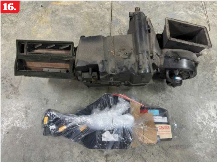
16. A simple side-by-side comparison shows the size difference and room you will gain under the dash.
