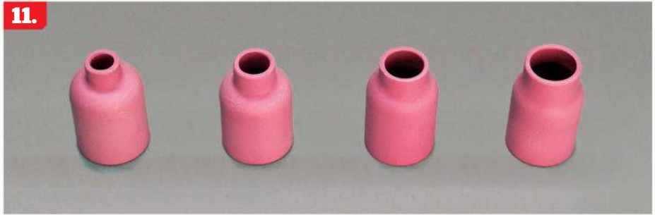
11. These are cups for a gas lens on a water-cooled #20 torch. They are shorter and wider than their air-cooled cousins.
