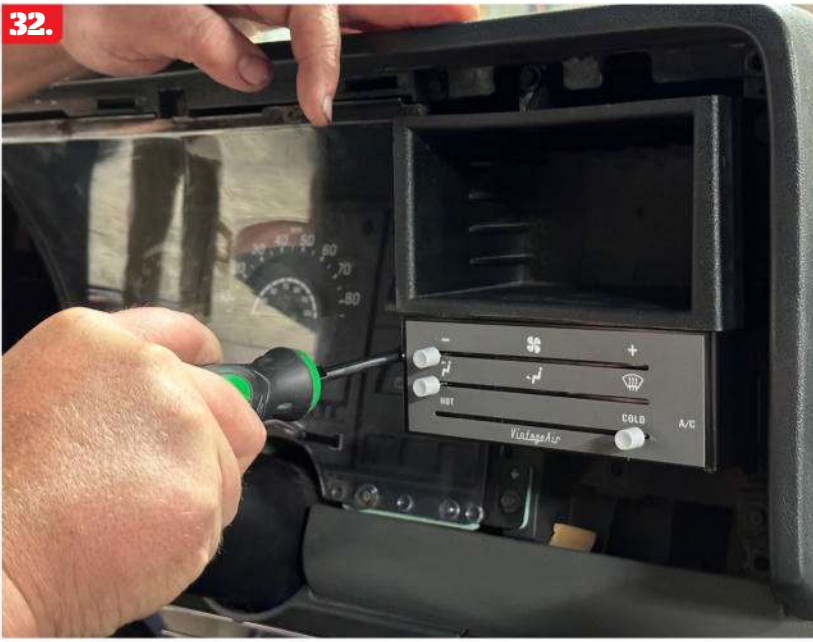
32. Mounting the control panel will be the easiest part of the whole installation—four screws in the stock location. Plug the harness off from the control to the module on the front of the evaporator.
