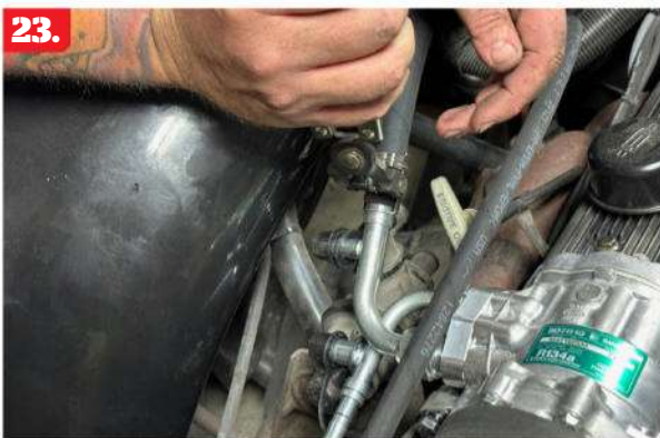
22-23. At this point, we decided to switch the crimp-style hoses supplied over to EZ-clip hoses to make our own at custom lengths. This was dictated because of the aftermarket fiberglass Slosh Tubs and adjustable suspension.
