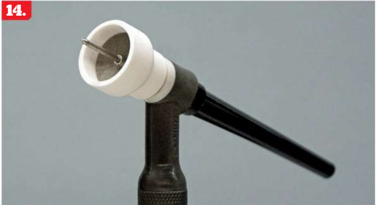
12. These are special "long reach" cups that aren't often needed, but they are available for special applications where the torch needs to be manipulated into deep recesses.
