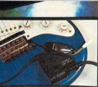
features a 'hex pickup' which lies under the bridge, and this supplies the pitch for the VG-8. Our review model was fitted so it can be used with any guitar. A certain manufacturer is even planning an with a GK-2A hidden inside the body.
