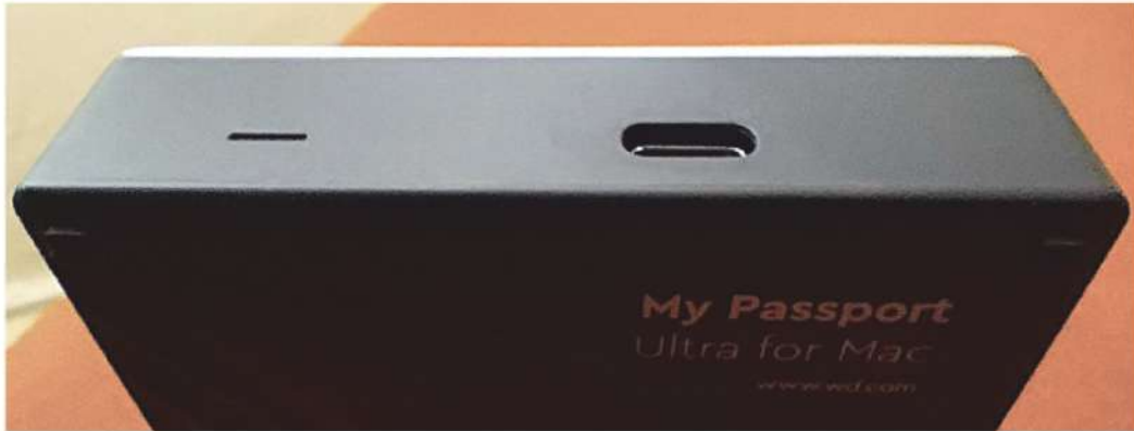
The Type-C connector and power-activity light are on the end of the My Passport Ultra for Mac.
