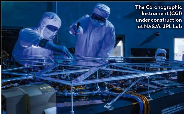
Roman's coronagraph uses a system of discs and flexing mirrors to sift starlight out of the images
