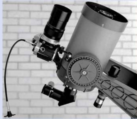
▲ A popular deep-sky setup in the 1980s: an Olympus OM-1 camera, telephoto lens and shutter release cable piggybacking a Celestron C5 telescope
