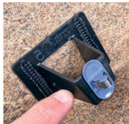
5 These metal clips on the carpeted inner might move during removal, so make sure you collect any that have come loose and refit them. They're quite durable and shouldn't break.
