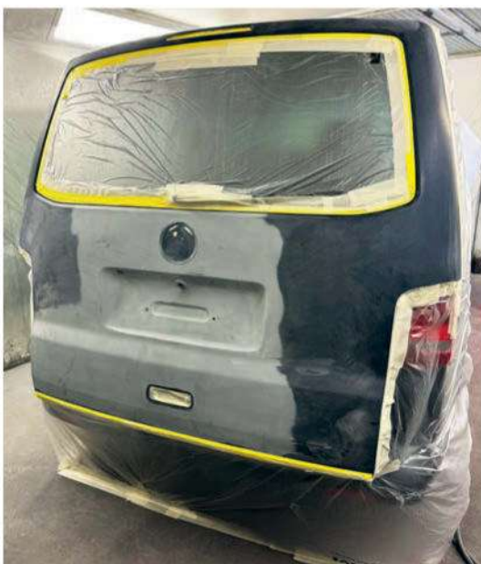
3 More work is required on the rear tailgate. Badges, numberplate and associated wiring are removed first, plus masking up of the tailgate handle and surrounding area. The panel paint is smoothed back with a 180-grit sander, then dents and the rust spot near the numberplate are tackled next.
