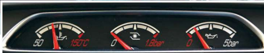
Dashtop mounted gauges for oil temperature, boost and oil pressure add a touch of visual drama.
