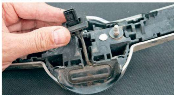
12 Unclip the electrical connector from the chrome trim as a first step. Make sure you don't fully shut the tailgate at this point.
