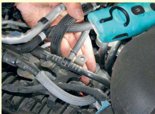
5 The air filter housing is in the nearside front corner of the engine bay. Attached to the induction pipe that's routed from it is a mass airflow (MAF) sensor.
