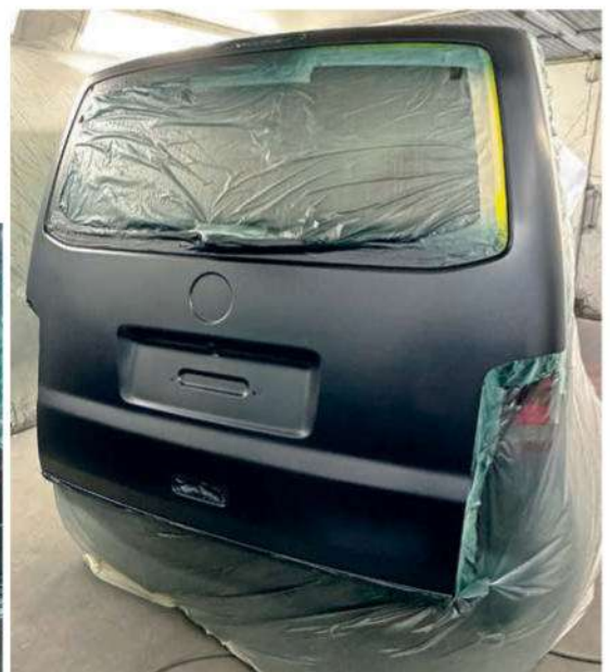
4 Once satisfied, the filler is smoothed and feathered into the surrounding paintwork, then a coat of primer is added. As you can see the whole tailgate isn't painted with primer, just the area that requires filler work.
