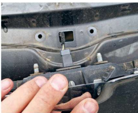
8 Two more 10mm nuts secure the chrome boot trim in place on either side of the lock's electrical connector. Remove these.
