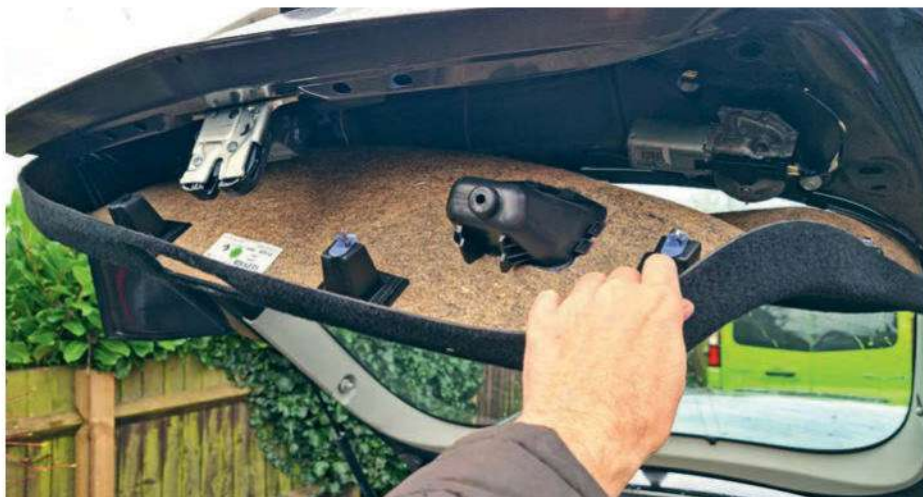
4 The tailgate inner lining can now be removed. It's only clipped in place so start by firmly pulling down the rearmost section and then remove it from the front slots.
