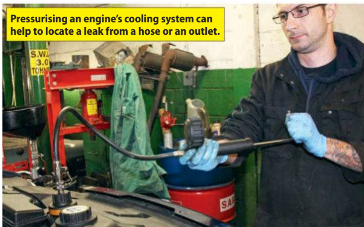
Test kit from Sealey includes an assortment of adaptors that replace a standard pressure cap to help pressurise a cooling system and look for leaks.
