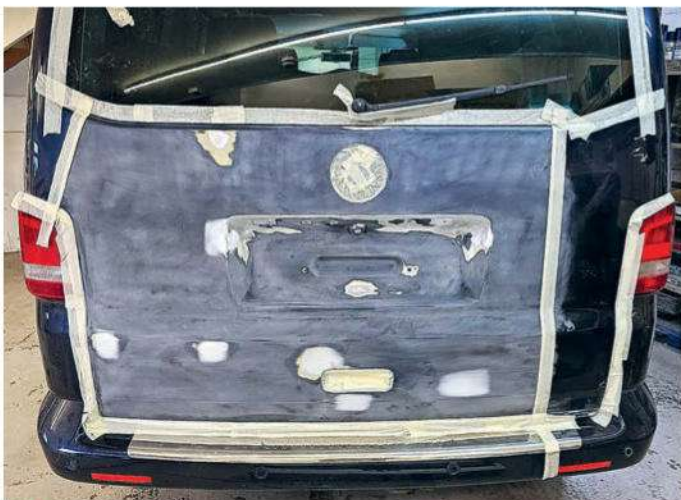
3 More work is required on the rear tailgate. Badges, numberplate and associated wiring are removed first, plus masking up of the tailgate handle and surrounding area. The panel paint is smoothed back with a 180-grit sander, then dents and the rust spot near the numberplate are tackled next.
