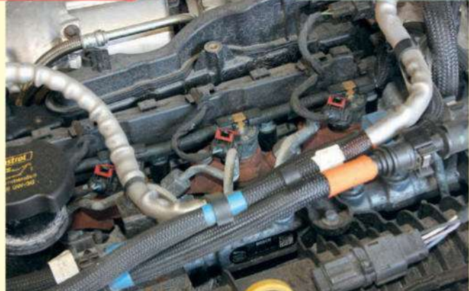
6 Removal of the top engine cover (it sits on locating pegs) and the soundproofing material underneath exposes the fuel injectors and more sensors.
