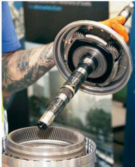
A32 The second gear set lifts out with the complete input shaft.
