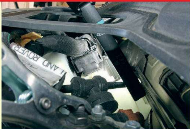
11 The ECU is located underneath the scuttle trim panel at the back of the engine bay. It can be seen if the panel for the battery (see Step 1) is removed.
