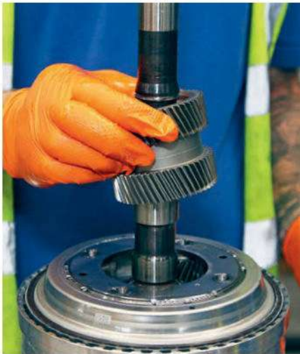
A31 With the sun gear assembly raised, the rest of the second planetary gear set is revealed.
