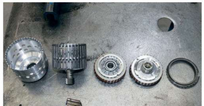
A35 ▶ Pictured from left-to-right, these components are: the basket, a drum with an integral sun gear that meshes with gear set 4, C clutch, D clutch and an annulus for the fourth gear set.
