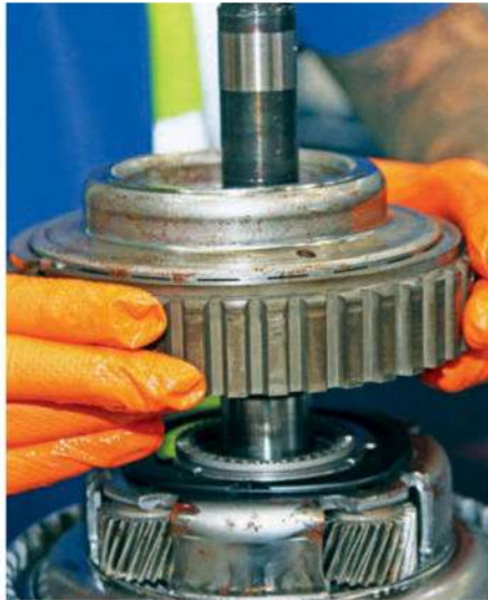
A29 Beneath the hub, pictured being lifted away, is the planetary gear assembly, that comprises the first gear set.
