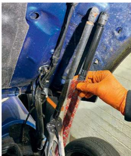
Check the length, use a screwdriver to lever out the clips then pop off the ball joints – easy!
