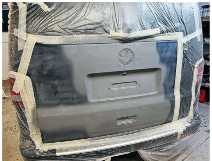
4 Once satisfied, the filler is smoothed and feathered into the surrounding paintwork, then a coat of primer is added. As you can see the whole tailgate isn't painted with primer, just the area that requires filler work.
