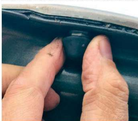
6 Next the fixings to the chrome boot trim need to be removed. To access the outermost ones, remove these rubber covers to reveal the nuts.
