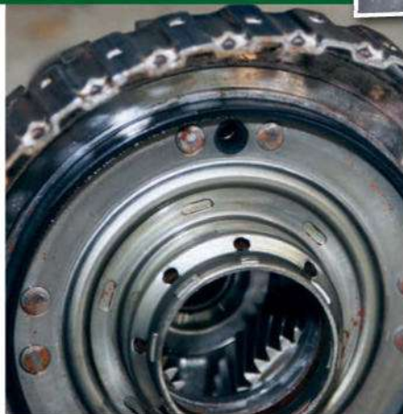
A39 The drum incorporating Gear Set 4 includes the integral hydraulic piston that squeezes the clutch packs together.
