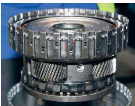
A36 ◀ The fourth gear set is positioned at the back of the gearbox. During this dismantling demonstration, the gearbox is mounted on a special stand, so you cannot see the output shaft.
