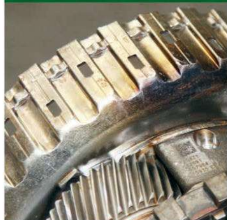
A38 The 'blueing' on the outer drum (which is not hardened from new, unlike the input shaft) indicates that the clutches have been slipping and overheating.
