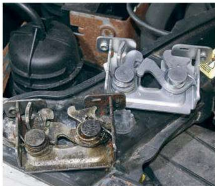
9 Comparing the old bonnet locking mechanism with the new one, they were clearly identical. We were relieved to discover we'd bought the right one.
