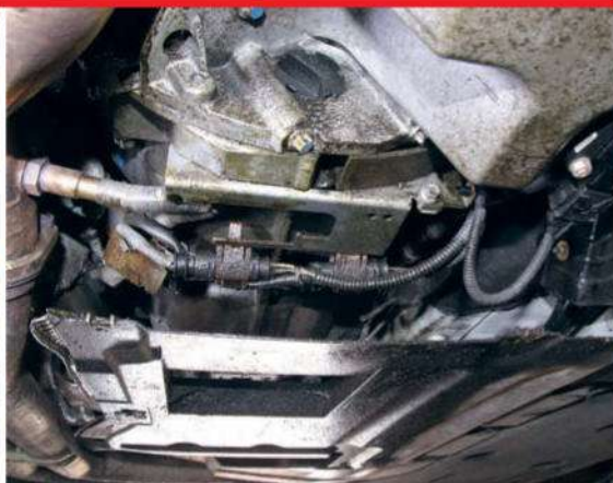
10 The end of the release cable was attached to the new locking mechanism, then the two were manoeuvred into the mount, the two Torx T30 screws fitted, and the other end of the cable reconnected. Flicking the latch over, the release lever opened it, so we shut the bonnet and opened it, this time with ease.
