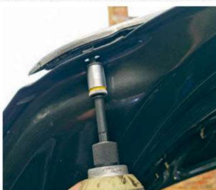
7 Remove the two outer 10mm nuts with either an impact driver or a 1/4-inch driver ratchet. Little force will be needed as they're only light duty fixings.
