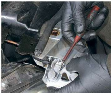
10 The end of the release cable was attached to the new locking mechanism, then the two were manoeuvred into the mount, the two Torx T30 screws fitted, and the other end of the cable reconnected. Flicking the latch over, the release lever opened it, so we shut the bonnet and opened it, this time with ease.
