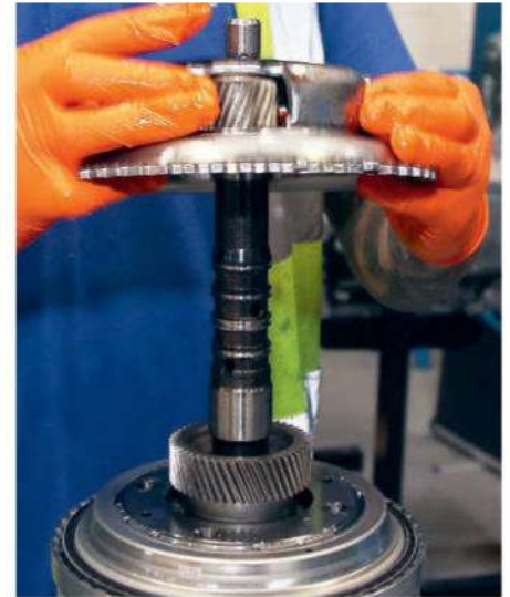
A30 Once the first gear set is lifted from the input shaft, the sun gear can be seen for the second gear set.
