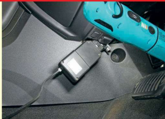
12 The EOBD port for connecting diagnostic equipment (or a dongle) is in the driver's footwell, close to the gearbox tunnel.
