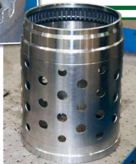
A40 As shown in Step A25, the components behind the oil drive/front cover are contained within a large basket, which is incredibly light and strong. However, it can be broken surprisingly easily by inexperienced repairs.
