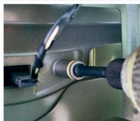
8 Two more 10mm nuts secure the chrome boot trim in place on either side of the lock's electrical connector. Remove these.
