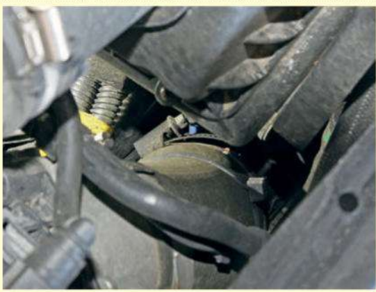
9 ◀ Across the front of the engine bay (behind the slam panel), there's the inlet manifold with a Manifold Absolute Pressure (MAP) sensor fitted. The plug next to it is blanked off in this case, so it's redundant.
