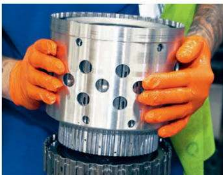
A31 With the sun gear assembly raised, the rest of the second planetary gear set is revealed.
