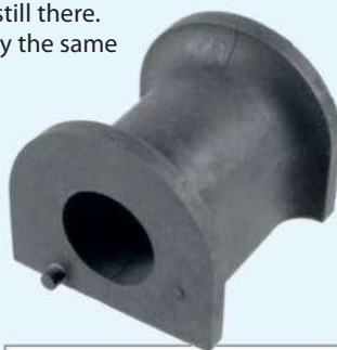
The anti-roll bar D-bush that may have gone hard allowing the knocking noise.
