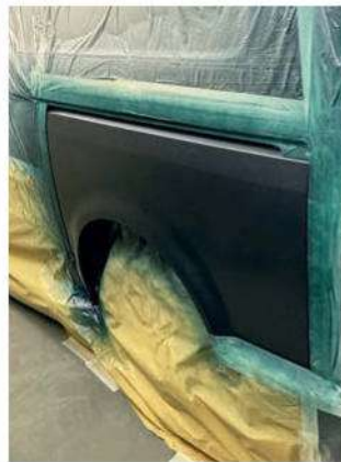
6 The first coat of Night Blue goes on the tailgate and rear arch section.
