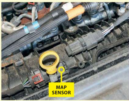
9 ◀ Across the front of the engine bay (behind the slam panel), there's the inlet manifold with a Manifold Absolute Pressure (MAP) sensor fitted. The plug next to it is blanked off in this case, so it's redundant.
