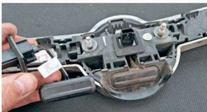
11 With the chrome trim section inverted and placed on the parcel shelf of the car, compare the old and new switches are compatible.
