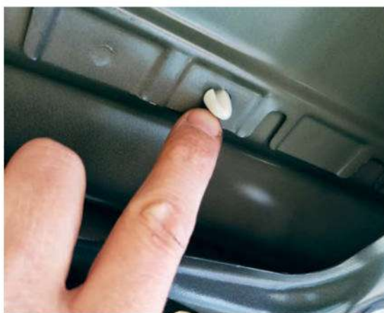
6 Next the fixings to the chrome boot trim need to be removed. To access the outermost ones, remove these rubber covers to reveal the nuts.
