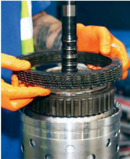
A28 Pictured is the second clutch pack (clutch B, which is also a brake) being lifted from the input shaft.
