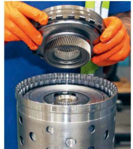
A33 The third planetary gear set's sun gear is then lifted out, followed by the third gear set.
