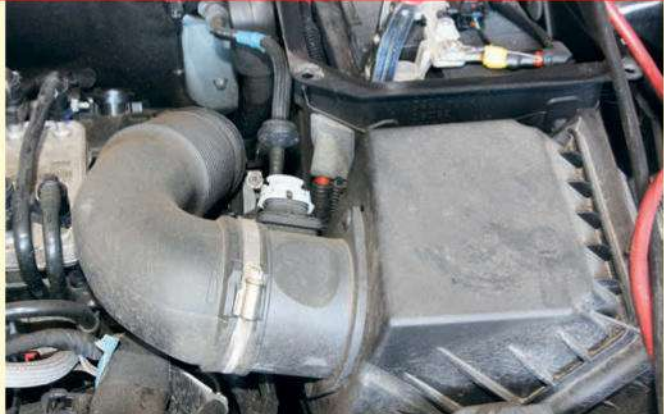
5 The air filter housing is in the nearside front corner of the engine bay. Attached to the induction pipe that's routed from it is a mass airflow (MAF) sensor.
