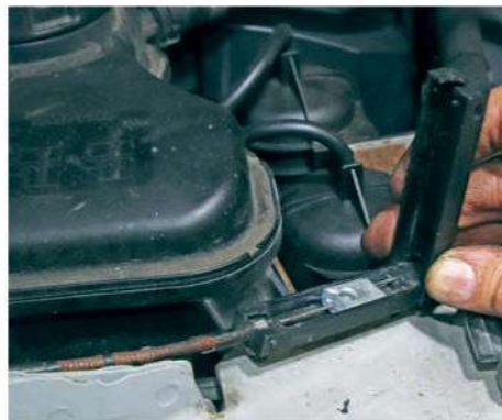
10 The end of the release cable was attached to the new locking mechanism, then the two were manoeuvred into the mount, the two Torx T30 screws fitted, and the other end of the cable reconnected. Flicking the latch over, the release lever opened it, so we shut the bonnet and opened it, this time with ease.
