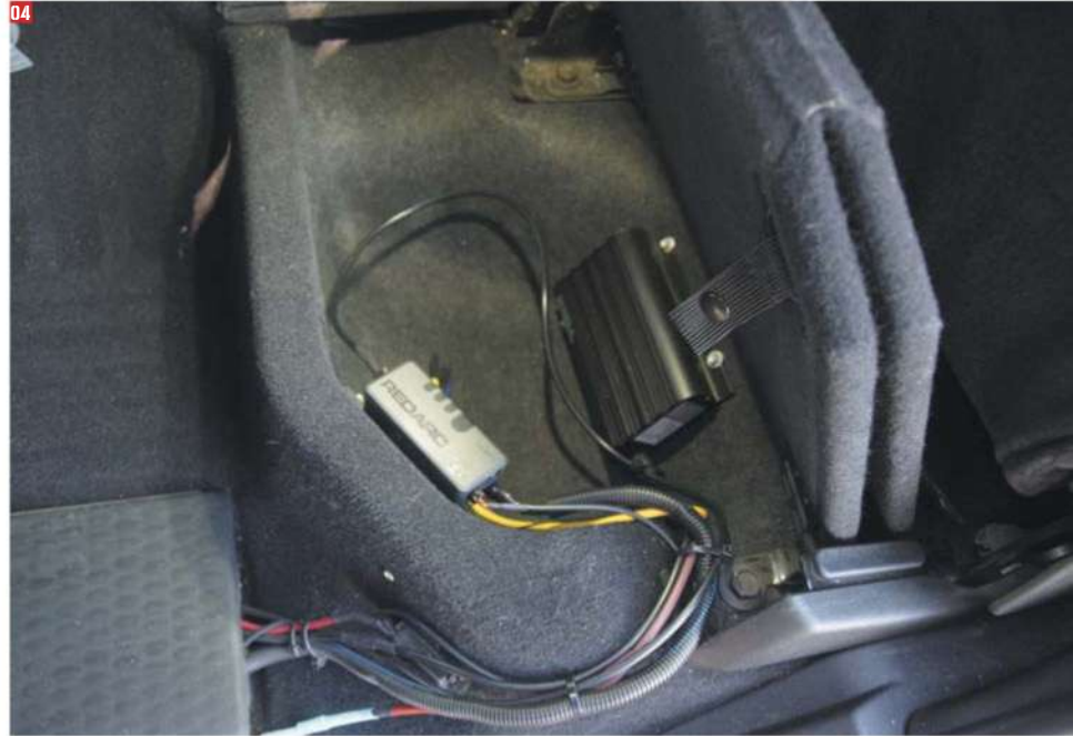
04. I mounted the REDARC smart battery monitor and the REDARC BCDC1225D in-vehicle dual battery charger under the rear seat of my RAM 1500. The wiring is mocked up to run to the battery in the underfoot storage. The directions that come with the battery monitor and the charger will be critical to ensuring proper installation using the correct wire gauge and length of various wires.
