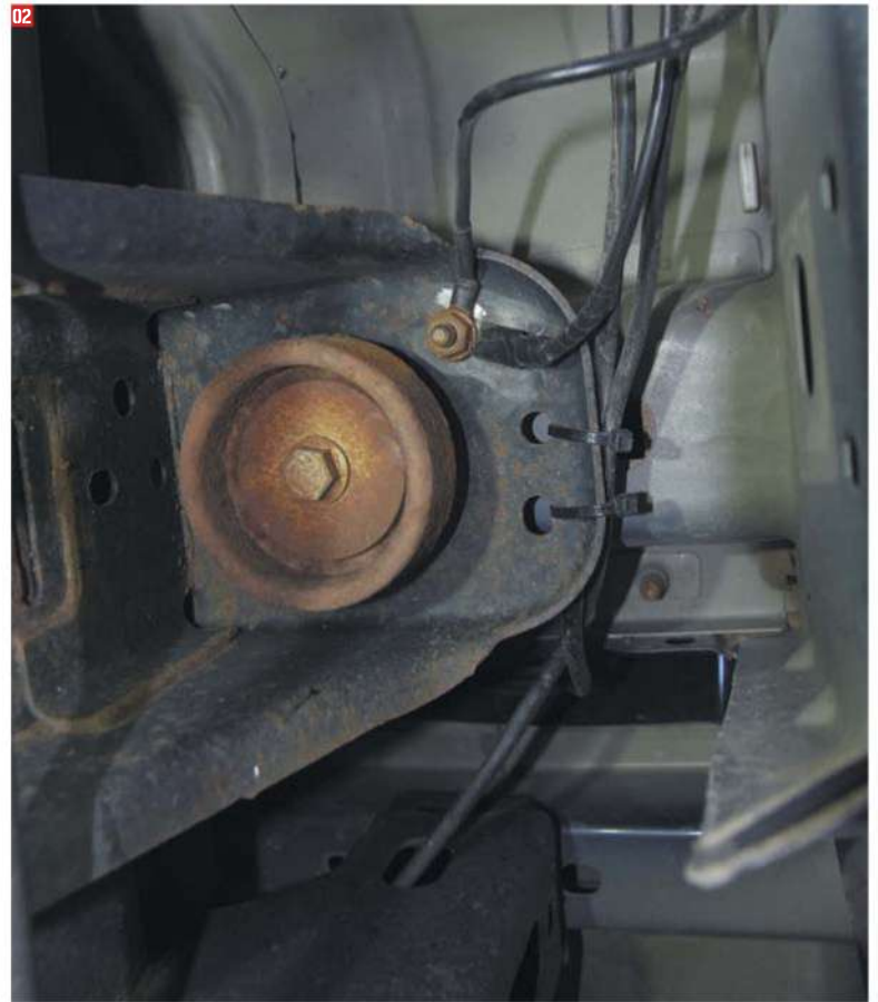
02. Make sure that you have cleaned the ground area to bare metal to ensure good contact. This is a critical step for wherever you choose to ground. Here, you can see I installed it near my driver-side seat.
