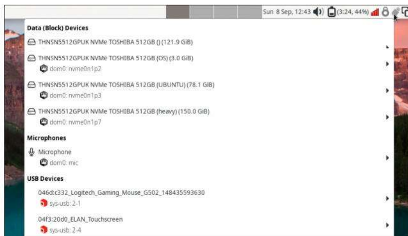
You can connect USB devices or internal storage to individual qubes. Microphones might be tricky.
