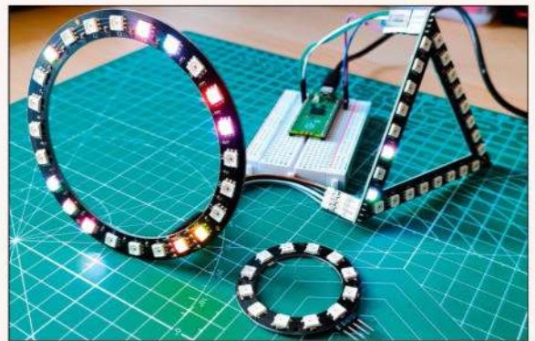
NeoPixels, DotStar and RGB LEDs are all different types of multicolour LEDs that we can control using just a few lines of MicroPython.
