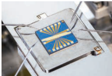
INBRAIN Neuroelectronics’s implants contain reduced graphene oxides (top). Graphenea uses monolayer graphene in its field effect transistors (bottom).
