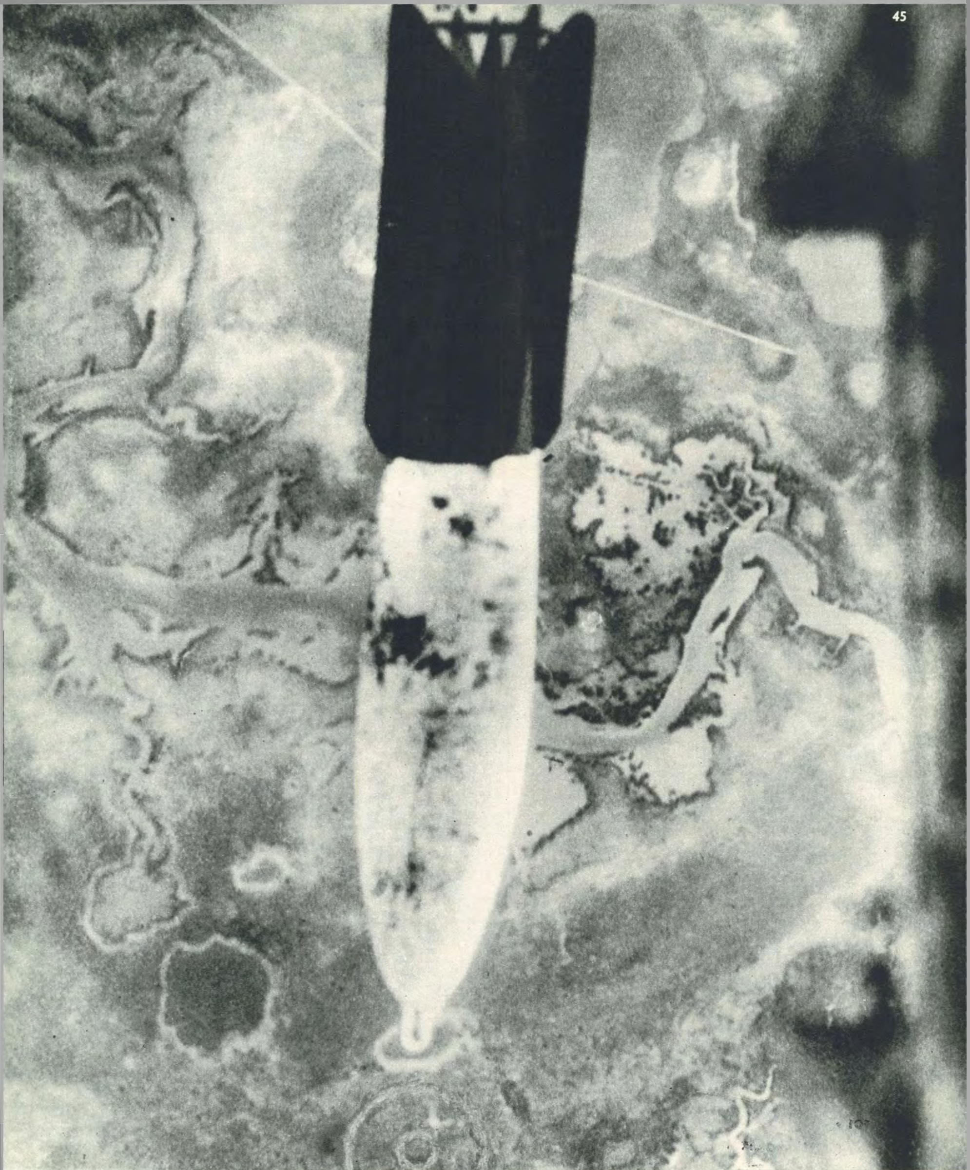
DESTRUCTION-BOUND Practice bomb leaving rack at 3,000-foot altitude and aimed for 100-foot circle target to test the plane bombarder's accuracy. (The Army's Closest Secret page 20)
