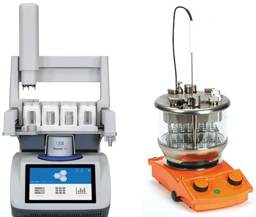
FIGURE 16.15 Laboratory stations for microwave-assisted organic reactions (CEM Explorer-24) and parallel synthesis (Radley's Greenhouse). View larger image
