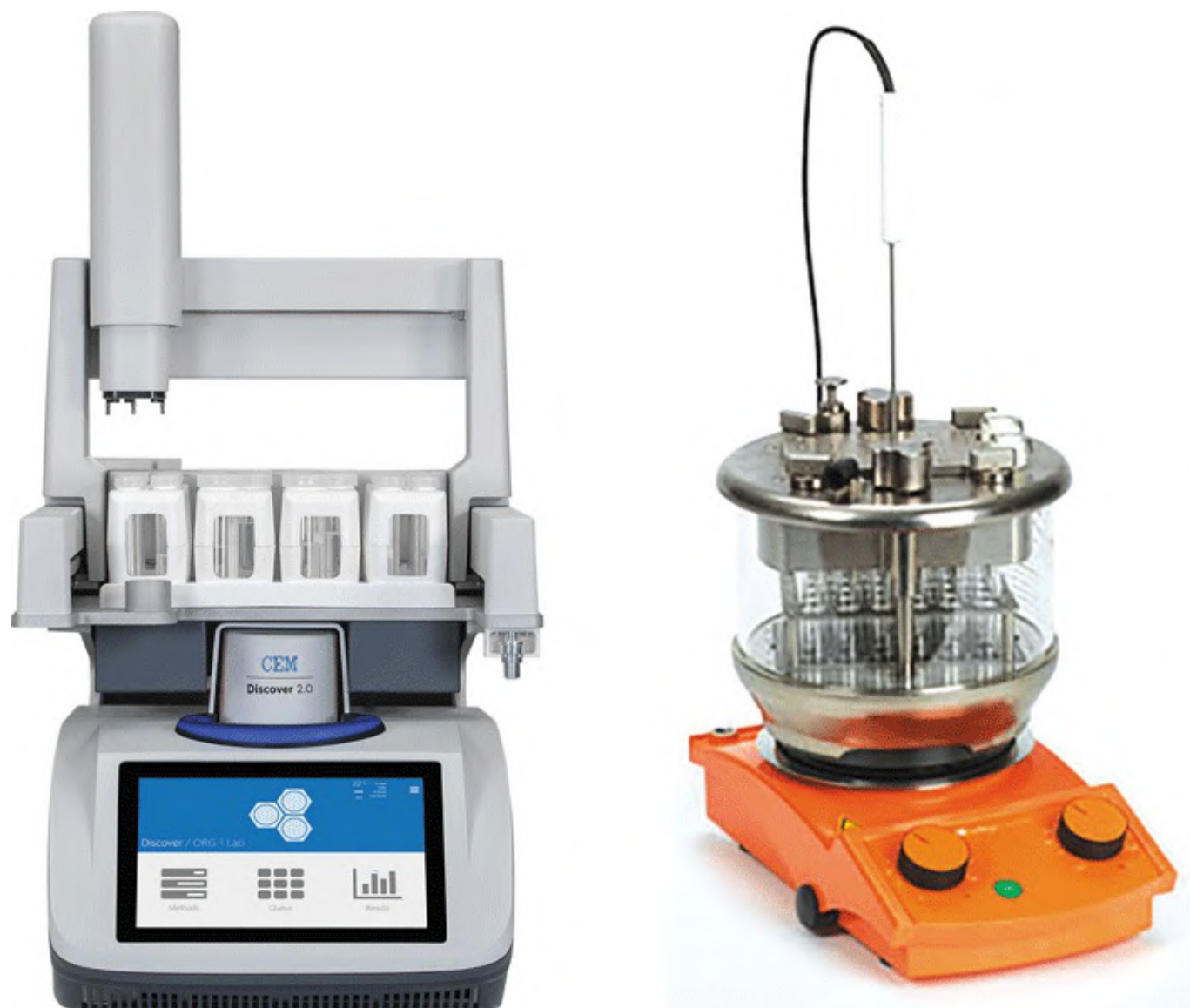
FIGURE 16.15 Laboratory stations for microwave-assisted organic reactions (CEM Explorer-24) and parallel synthesis (Radley's Greenhouse). Back to text
