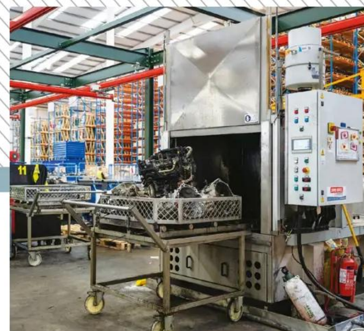
Engines and gearboxes being loaded into the engine washer
