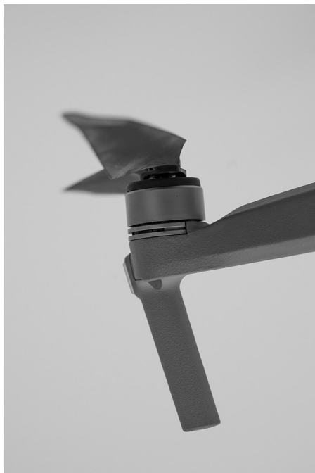
FIGURE 6.3 Brushless electric motor in drone.
