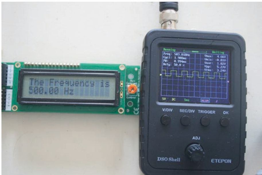
Figure 7-4. The 500Hz measurement using the sprintf function
