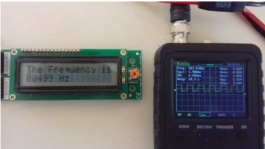
Figure 7-3. The display of a 500Hz square wave
