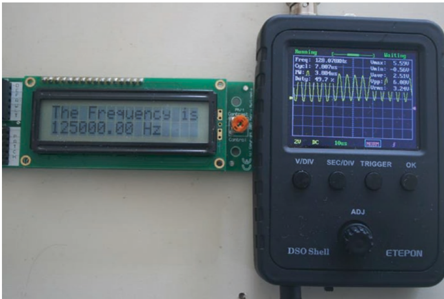
Figure 7-5. The 125kHz measurement using the sprintf function
