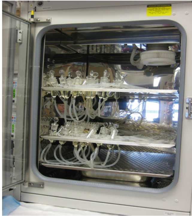
Fig. 5 Flow loop systems connected to the perfusion bioreactor
