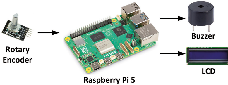
Figure 4.49: Block diagram of the project.
