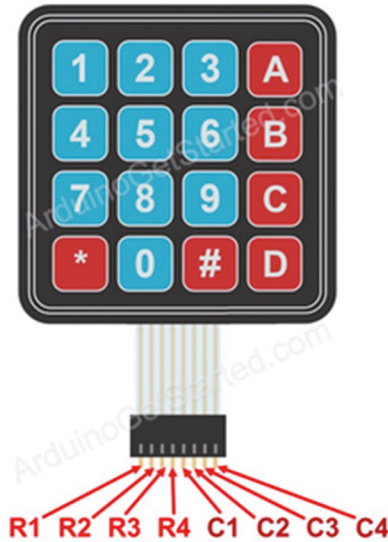
Figure 4.42: Pin configuration of the 4x4 keypad.
