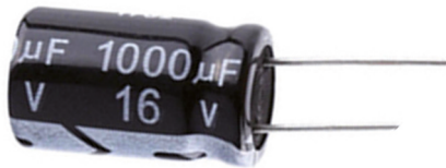
Figure 3.9: Electrolytic capacitor marking.
