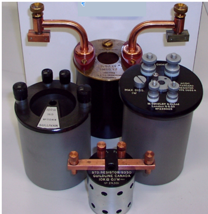
Figure 3.9. Resistance standards held at the National Physical Laboratory (NPL) England. Values available for calibration purposes range from 100 \mu\Omega to 1 G \Omega , with uncertainties of less than 1 ppm. Note the use of four terminals, two to carry a current and two to measure a voltage, thereby eliminating the resistance of the terminals. (Courtesy of the NPL.)
