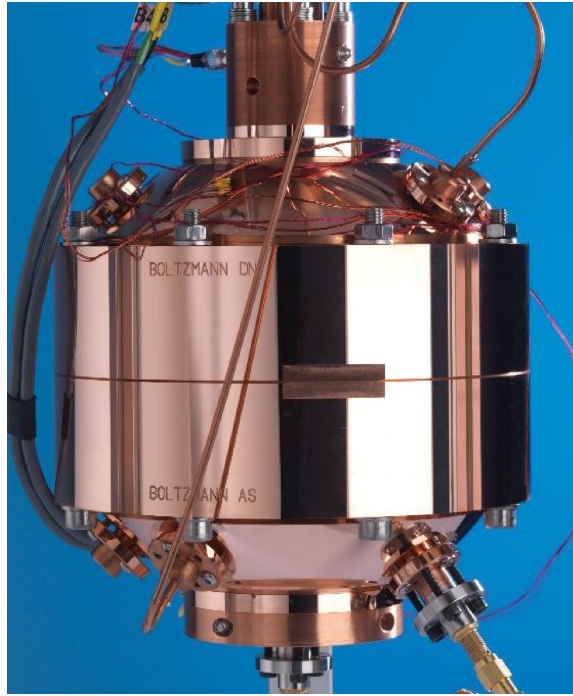
Figure 4.5. The NPL quasi-spherical acoustic resonator, made of diamond-turned copper, in which the Boltzmann constant was measured with uncertainties of less than one part per million, and, the quantity T-T_{90} was determined between 118 K to 303 K, in both cases, with the lowest uncertainties ever attained. Courtesy of NPL.
