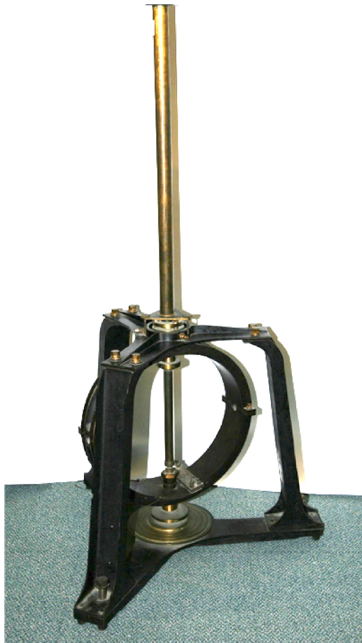
Figure 3.3. Redesigned rotating coil apparatus used by Lord Rayleigh to determine the value of the ohm in absolute units. Its rate of rotation was controlled and measured with the aid of a stroboscopic disc attached above the pulley (see figure 3.4). Suspended in the vertical tube at the centre of the coil is a small magnet whose deflection from the magnetic meridian was measured by the deflection of a light beam reflected from a mirror attached to the suspension above the magnet. (Courtesy: the Cavendish Laboratory, University of Cambridge.)
