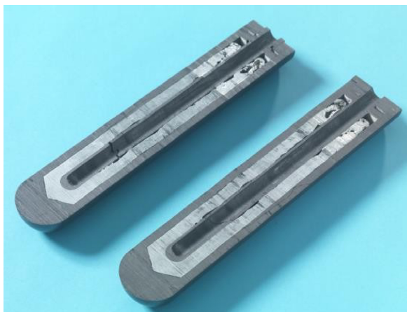
Figure 4.2. Section of a fixed point used for thermometry calibration.
