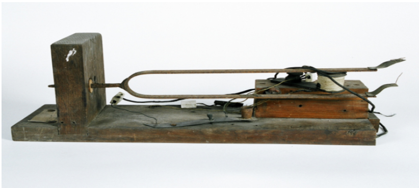
Figure 3.5. An electrically maintained tuning fork of the type used by Rayleigh to determine the rate of rotation of the coil. A dc voltage from a battery provides a current to the electromagnet (shown here with a white winding), which attracts the prongs of the fork. The circuit includes one of the prongs from which a wire is arranged to dip into mercury contained in a thimble (near the centre of the baseboard). As the fork vibrates, the circuit is opened and closed by this device, thereby providing an ac driving voltage to maintain the fork's vibrations. The stroboscopic disc is viewed through shutters (not shown here) attached to the ends of the fork. When a specific ring on the disc appears stationary, its frequency of rotation is some multiple of the fork's vibrational frequency.
