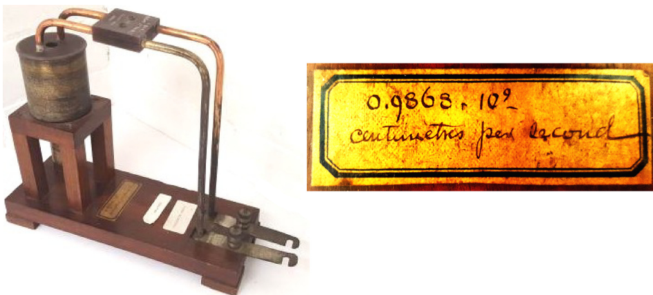
Figure 3.1. An early standard resistor with a value of very nearly 1 ohm expressed in terms of a velocity as seen on its label (courtesy of the University of Leeds Museum of History of Science, Technology and Medicine).
