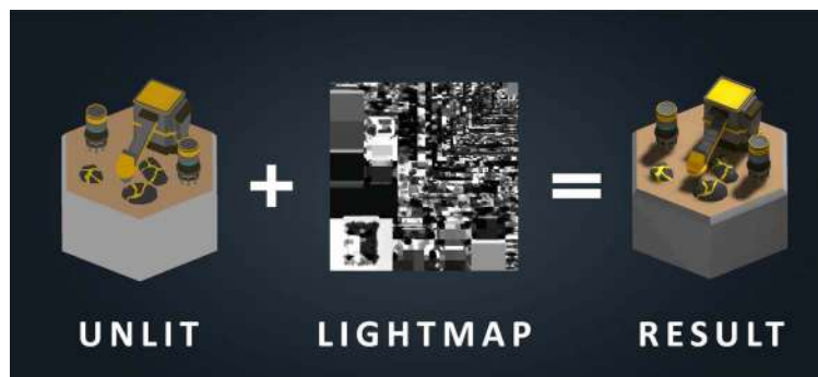
Figure 12.39: Left, a scene with no lighting; middle, a lightmap holding precalculated data from that scene; and right, the lightmap being applied to the scene
