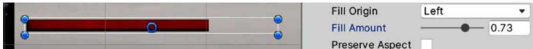
Figure 15.24: The Fill Amount slider, cutting the image width to 73% of its size
