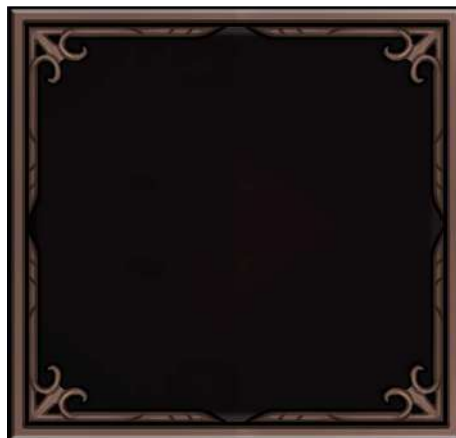
Figure 15.14: Optimized 9-slices background. The middle part will be a 1px strip of pixels that will expand
