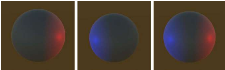
Figure 12.2: Left image, first draw call of a sphere affected by two lights in Multi-Pass; middle image, second draw call of the sphere; and right image, the combination of both draw calls
