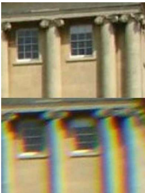
Figure 13.7: Image without chromatic aberration (top) and the same image with chromatic aberration (bottom)
