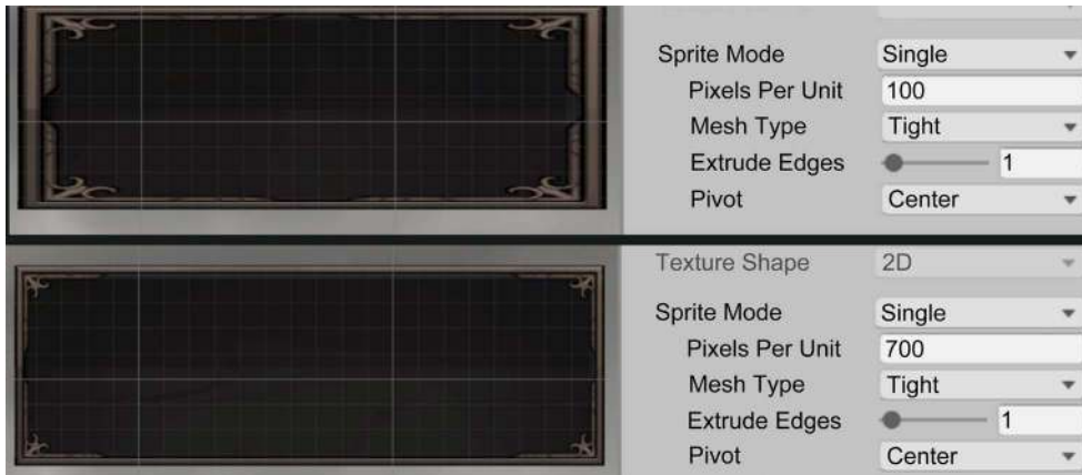
Figure 15.30: On top, a large 9-sliced image in a small RectTransform component, which is small enough to shrink the corners, and at the bottom, the same image with Pixels Per Unit set to 700
