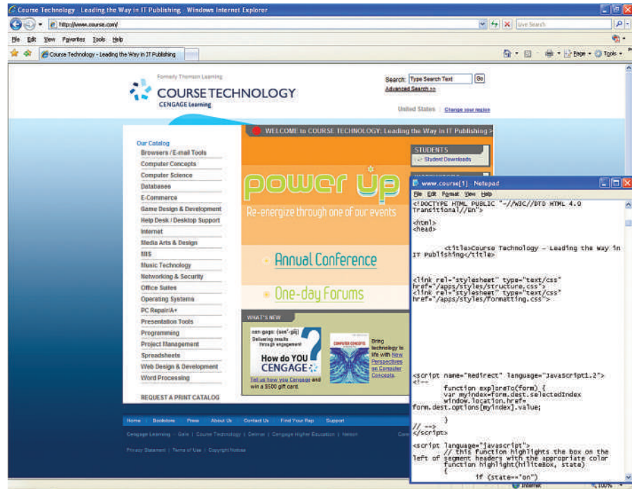
Figure 6.16 Sample Hypertext Markup Language Shown on the left of the screen is a document, and at the right are the corresponding HTML tags.
