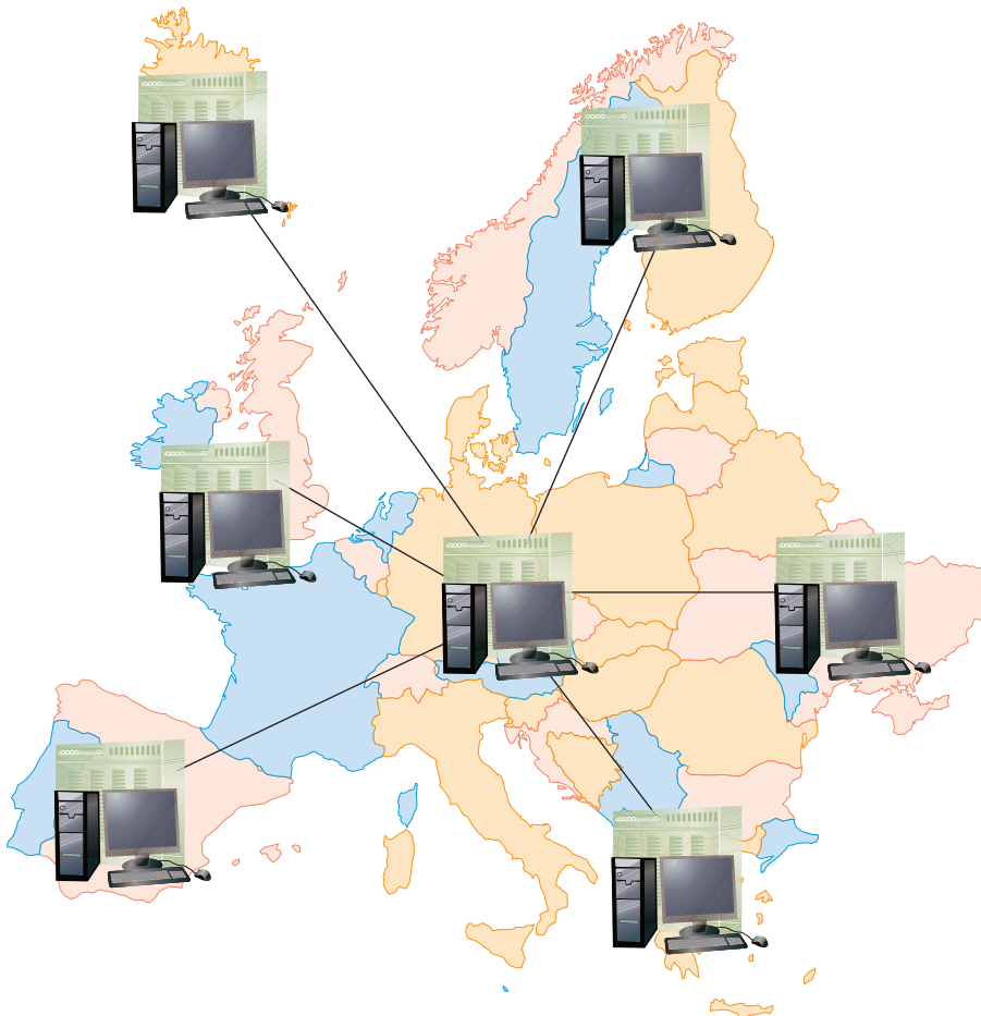
Figure 6.9 A Wide Area Network WANs are the basic long-distance networks used around the world. The actual connections between sites, or nodes, might be any combination of satellites, microwave or cabling. When you make a long-distance telephone call or access the Internet, you are using a WAN.
