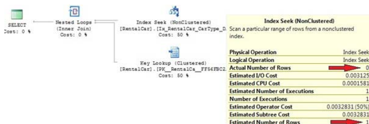
Picture 10: Improved execution plan with filtered indexes
