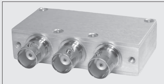
Mini-Circuits ZP-3LH+ Mixer: 0.15–400 MHz, 4.8 dB conversion loss, +10 dBm LO, 50 dB LO-RF isolation, 45 dB LO-IF isolation. Courtesy of Mini-Circuits® ( www.minicircuits.com ).
