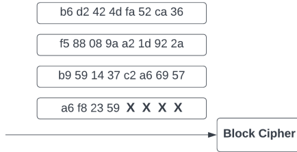
Figure 5.3 Example: x denotes padding bytes in the last block for a cipher with a block size of 8 bytes
