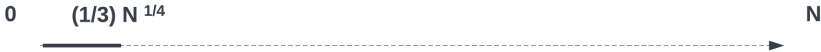
Figure 7.21 If d < \frac{1}{3}n^{\frac{1}{4}} , it can be efficiently found in convergents of \frac{e}{n}
