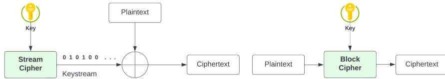
Figure 5.4 Stream ciphers generate a keystream which is subsequently XORed to encrypt, block ciphers directly output the ciphertext after encryption.
