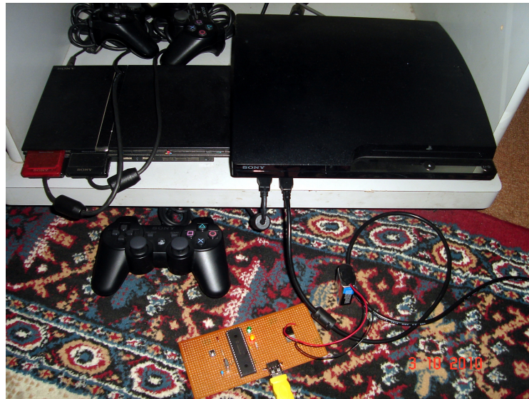
Figure 8.8 October 2010: My struggles with USB glitching to run unauthorized code on the PS3. The ECDSA vulnerability had not yet been discovered.
