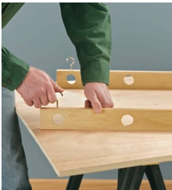
1. After you have drilled one-inch holes in each stretcher, insert J-hooks at each end.
