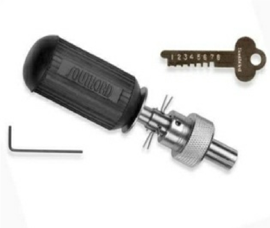
Fig: A Tubular Lock with a Decoder (Top Right) and a Tension Wrench (Bottom Left)
