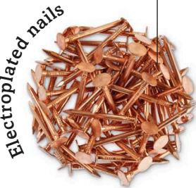
Copper coating on steel slows down corrosion.
