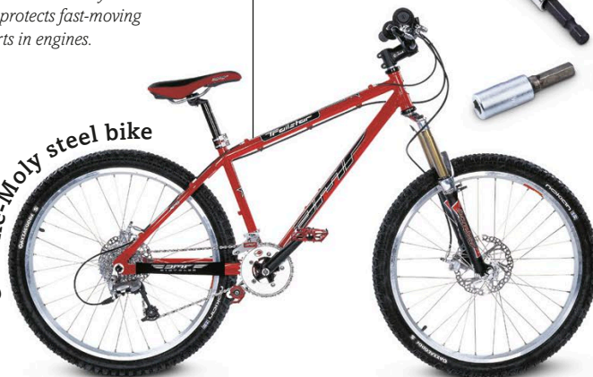
This lightweight but stiff frame is made from a steel containing molybdenum and chromium.
