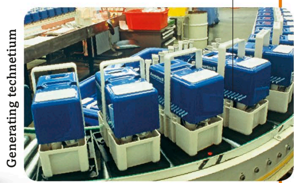
This box contains radioactive molybdenum, which breaks down into technetium.
